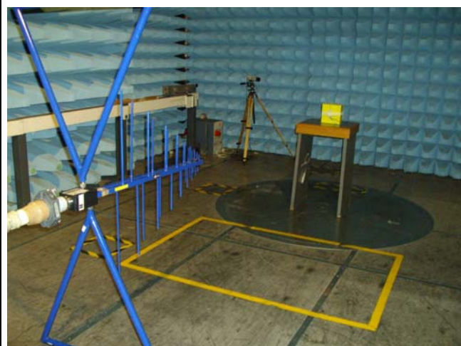
PHOTO N°2 – Emission radiated setup
