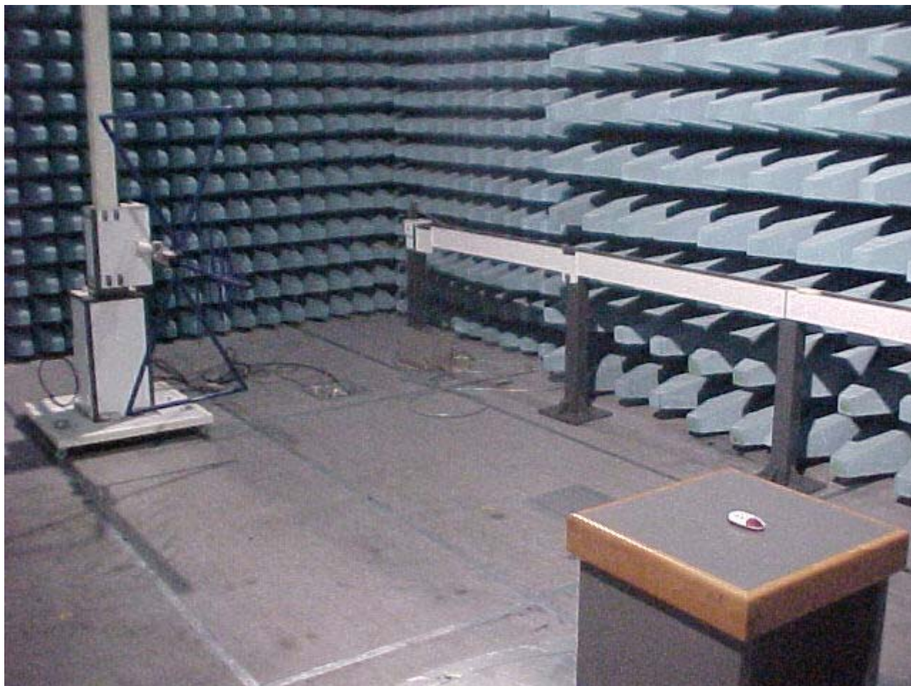
PHOTO N° 3 – SET-UP FOR RADIATED EMISSION TEST
