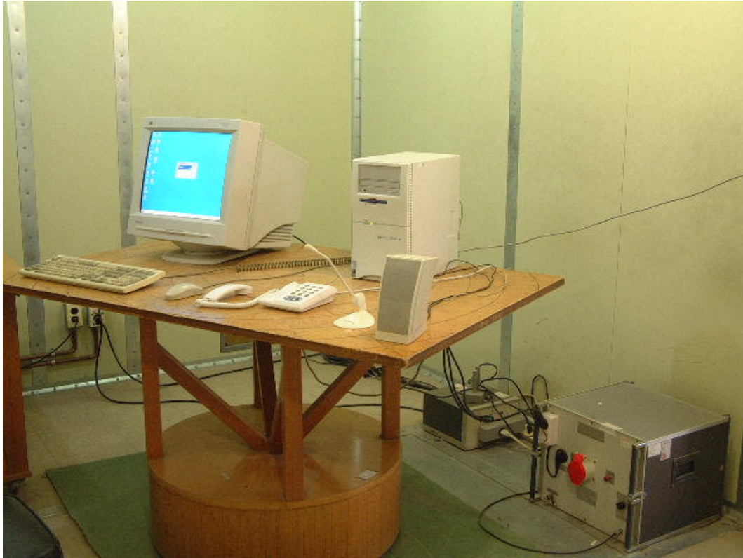
LINE CONDUCTED SETUP PHOTOGRAPH - FRONT VIEW
