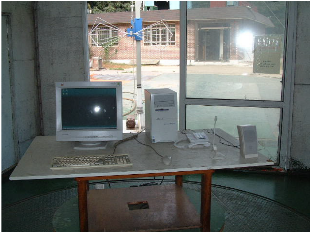
RADIATED EMISSION SETUP PHOTOGRAPH - FRONT VIEW ( 30 - 300 MHz )
