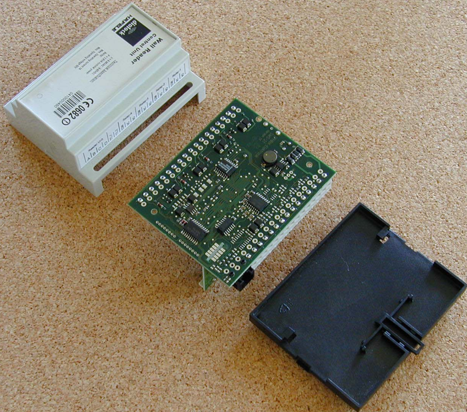
WT2000T Control Box apart (top)
