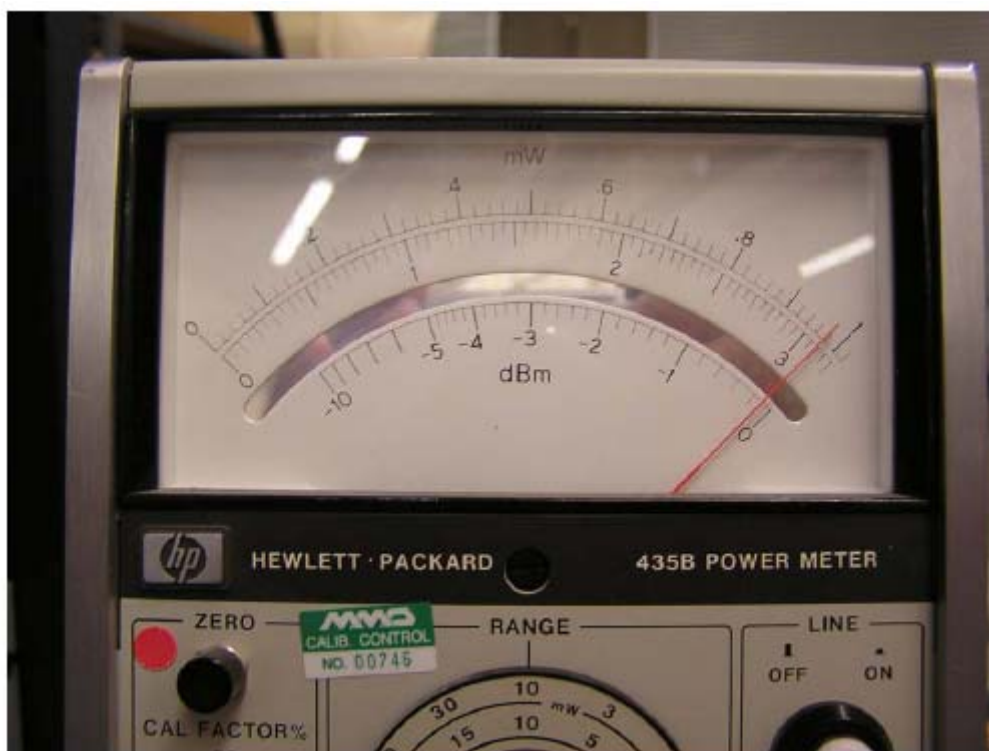
Meter indicating 9.9 dBm for visual RF Power Output
