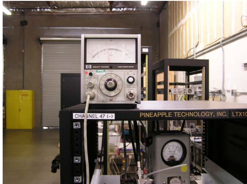
Fig. 1 Meter indicating -3.75 dBm for visual RF Power Output
