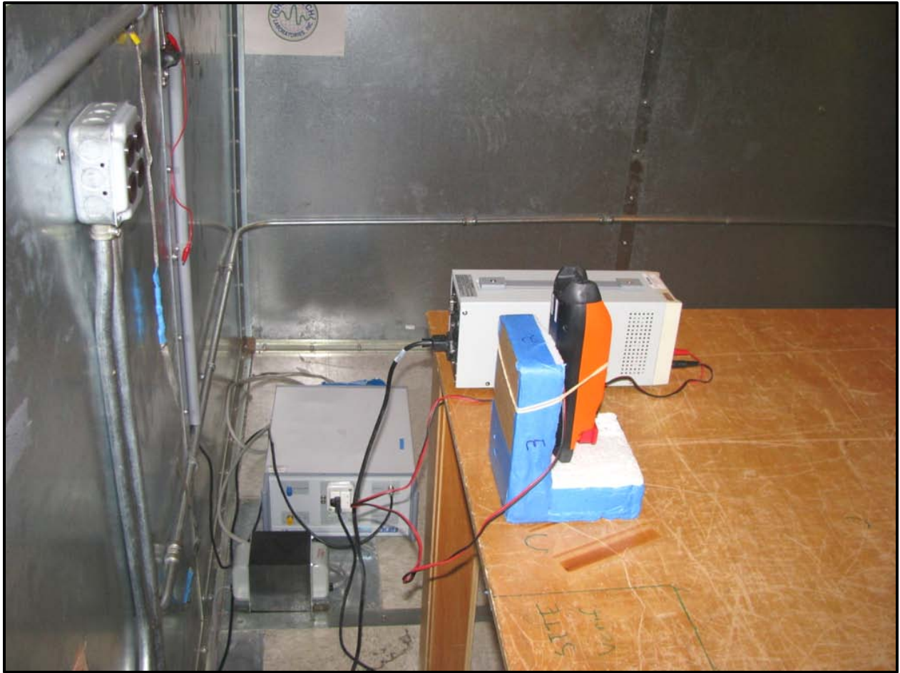
Photograph 4: Conducted AC Emissions - Rear View in Typical Host
