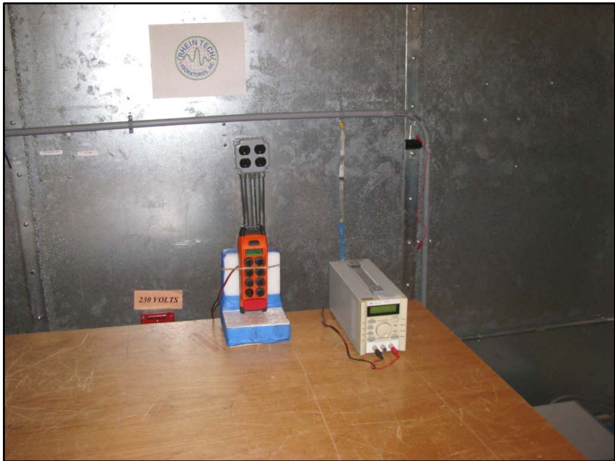
Photograph 3: Conducted AC Emissions - Front View in Typical Host
