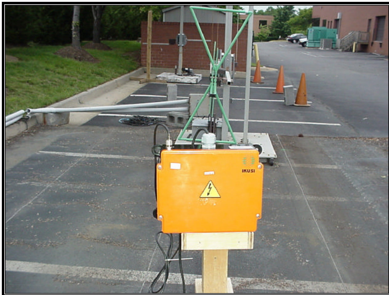
Photograph 3: Radiated Emission Front View –Unattached Antenna Configuration
