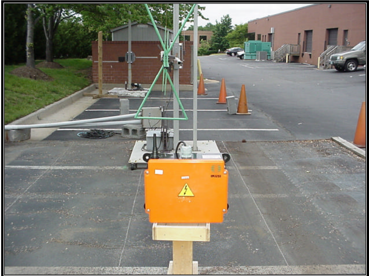
Photograph 1: Radiated Emission Front View – Attached Antenna Configuration
