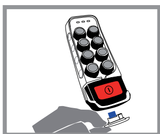
Remove the EEPROM in order to disable the transmitter
