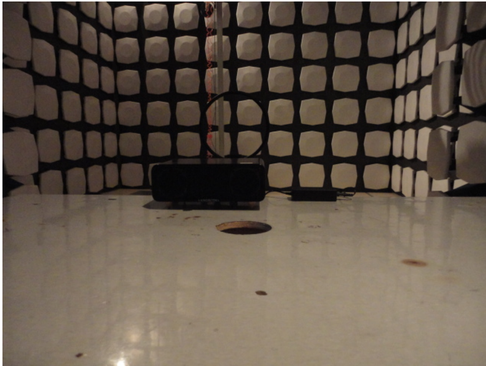
2: Radiated emission (30-1000MHz)
