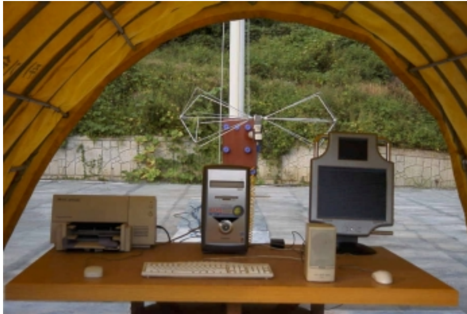
Photograph 1 : Setup for radiated Emissions
