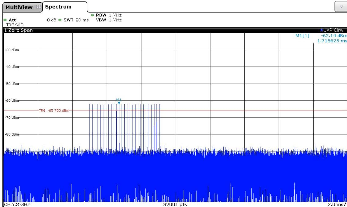
Radar test signal used in 5470-5725 MHz band (detection threshold calibration plot)
