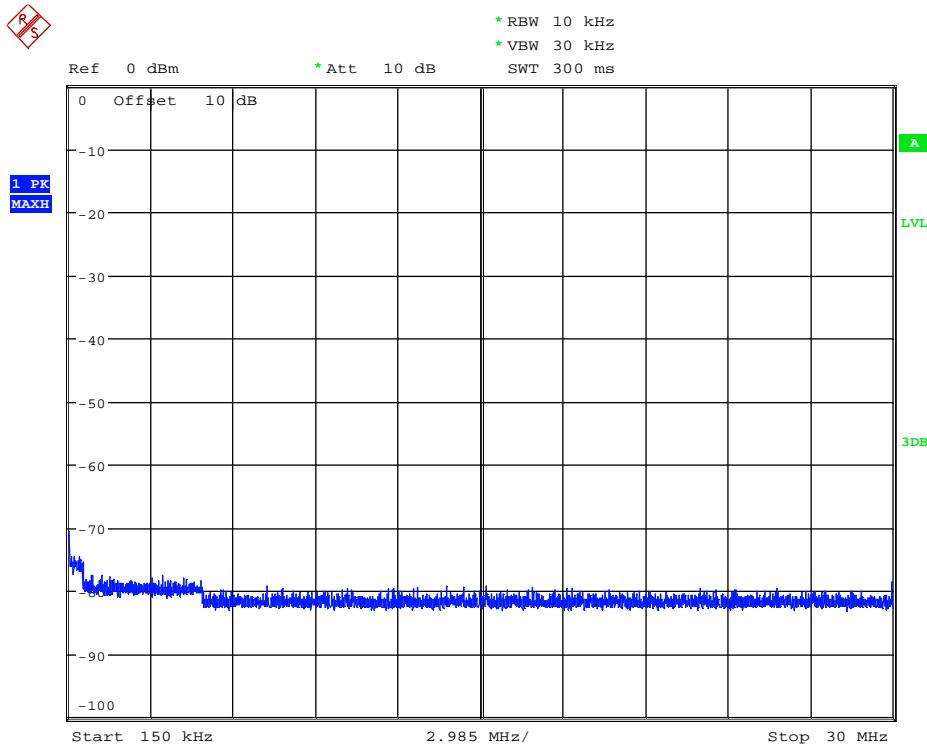
136117\_30M-1G\_allModesWLAN\_b\_1.wmf: conducted spurious emissions (operation mode 1):
