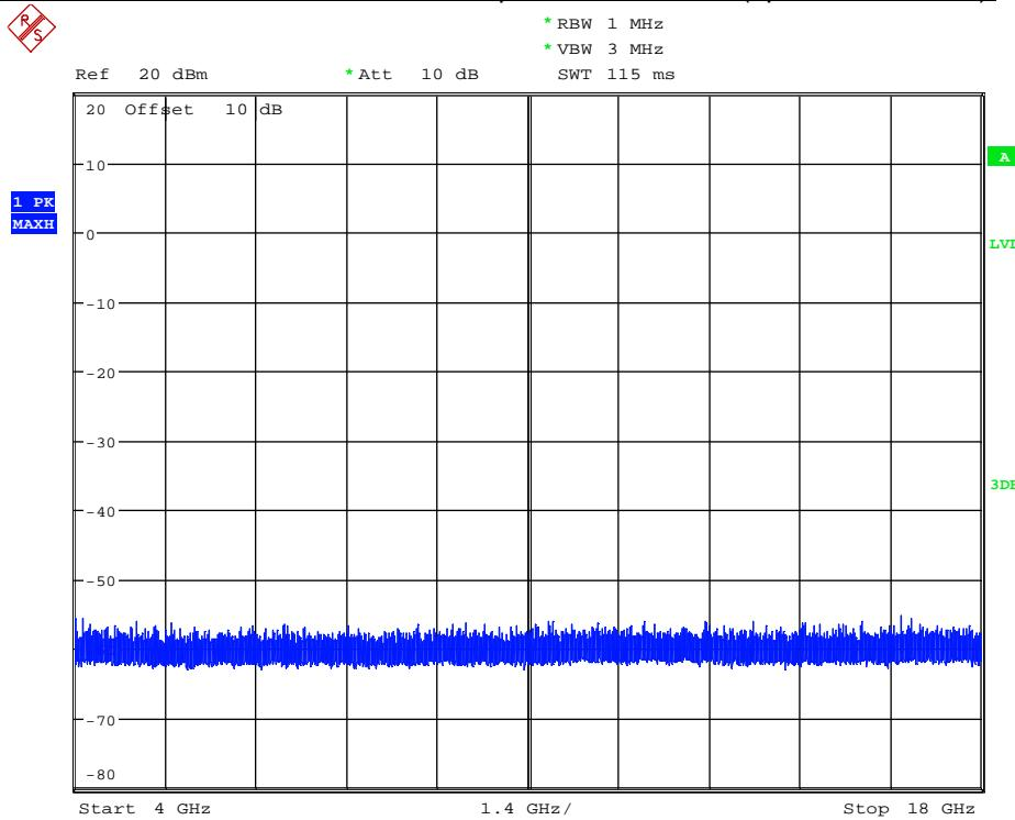
136117\_SpurEmiss18-26,5G\_n20\_6.wmf: conducted spurious emissions (operation mode 5):
