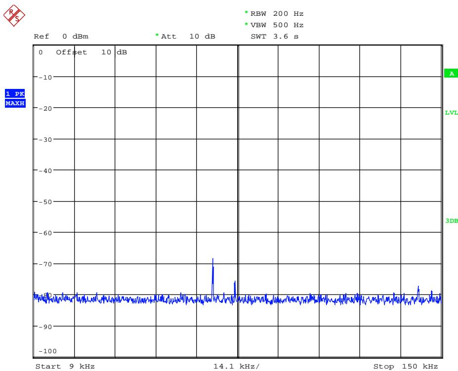
136117\_150k-30M\_allModesWLAN\_b\_1.wmf: conducted spurious emissions (operation mode 1):
