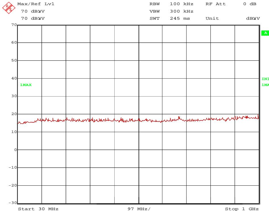
**Transmitter operates at the lower end of the assigned frequency band (operation mode 1)**
