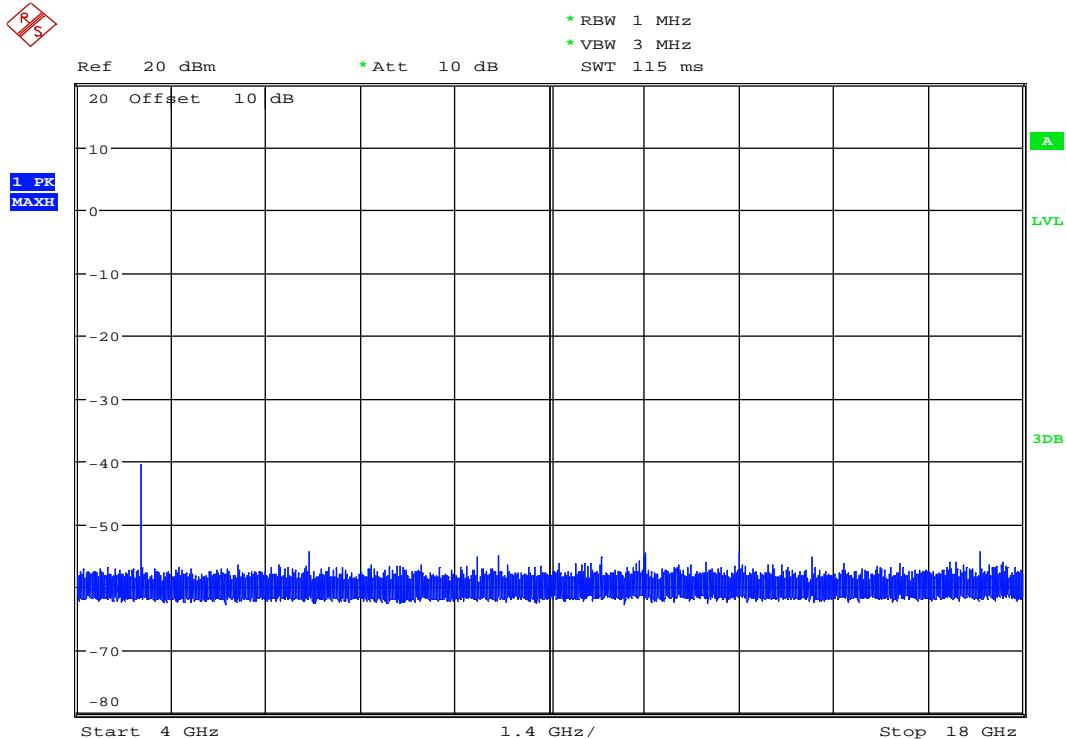
136117\_SpurEmiss18-26.5G\_BT\_DH5\_BT79.wmf: conducted spurious emissions (operation mode 5):
