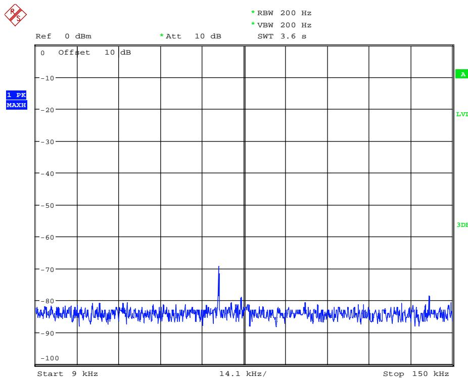
136117\_SpurEmiss150k-30M\_BT\_DH5\_BT79.wmf: conducted spurious emissions (operation mode 3):
