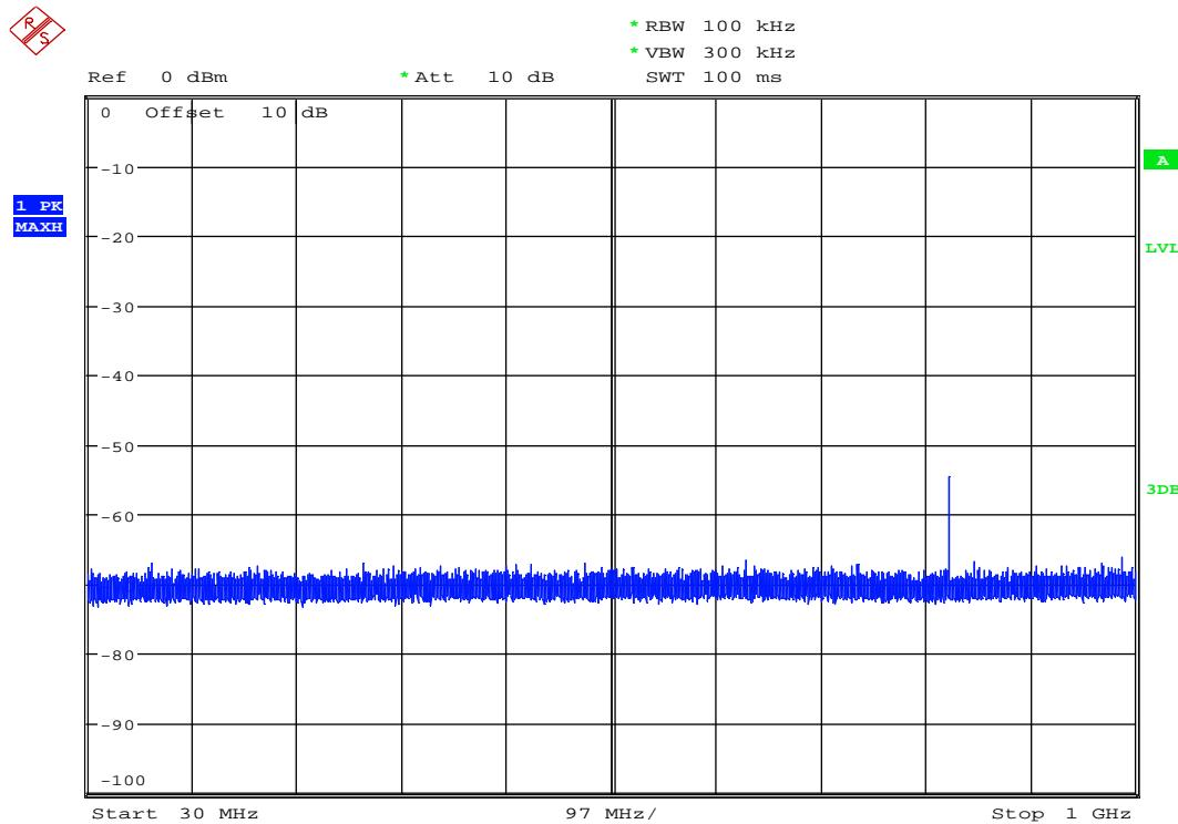
136117\_SpurEmiss1-4G\_BT\_DH5\_BT79.wmf: conducted spurious emissions (operation mode 3):
