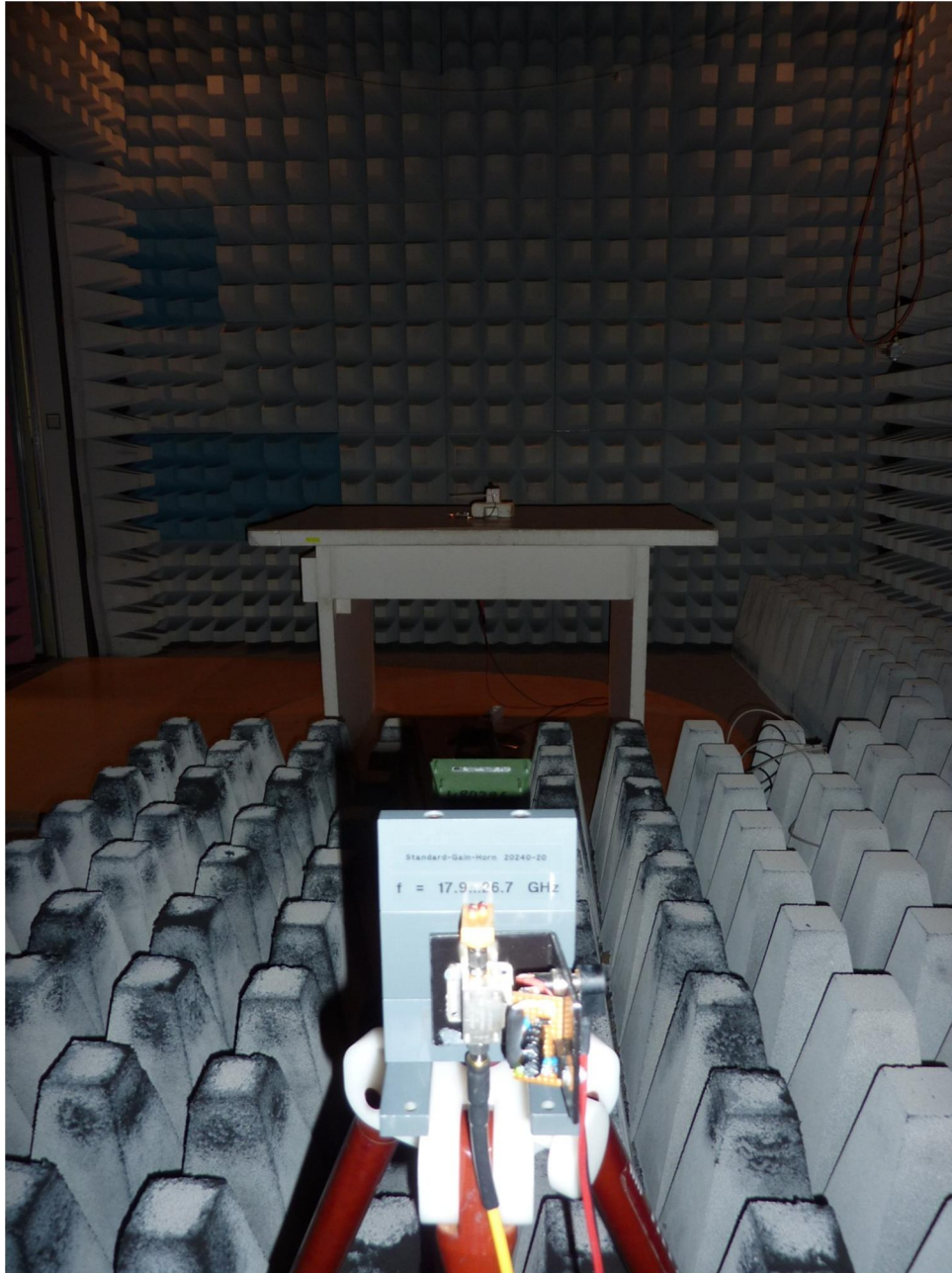
124266_4.JPG: Test setup fully anechoic chamber
