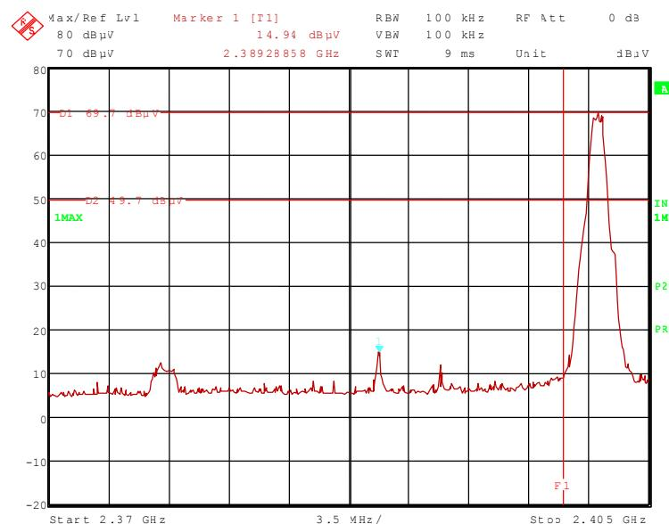
111592\_138.wmf: Radiated band-edge compliance, lower band edge, hopping on (operation mode 9):
