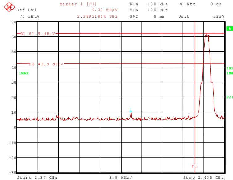
111592\_134.wmf: Radiated band-edge compliance, lower band edge, hopping on (operation mode 9):
