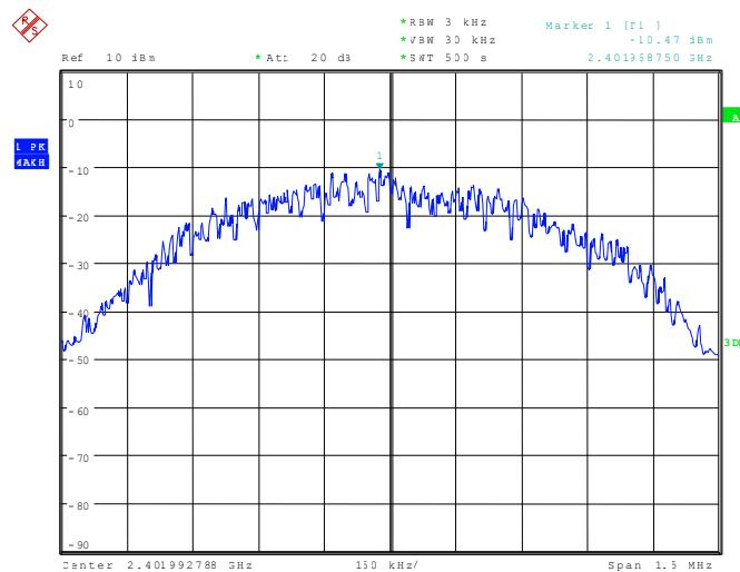
111592\_314.wmf: Power spectral density at the middle of the assigned frequency band:
