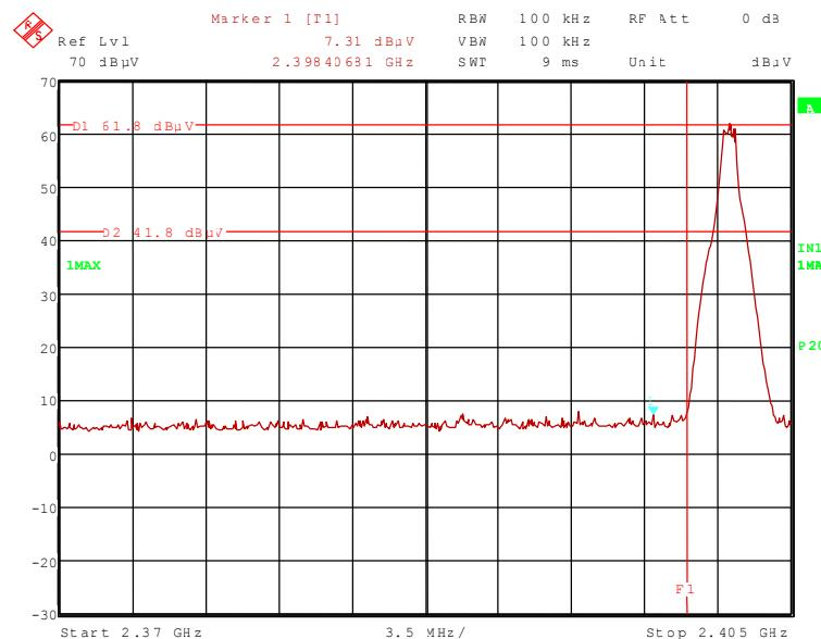
111592\_137.wmf: Radiated band-edge compliance, lower band edge, hopping on (operation mode 9):
