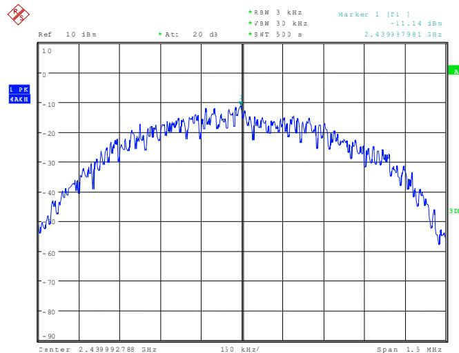
111592\_313.wmf: Power spectral density at the upper end of the assigned frequency band:
