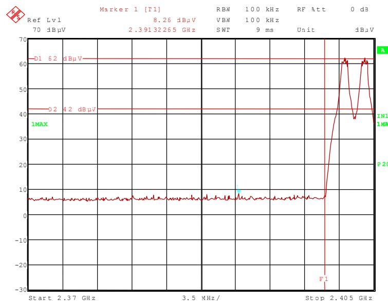
111592\_82.wmf: Radiated band-edge compliance, upper band edge, hopping off (operation mode 8):
