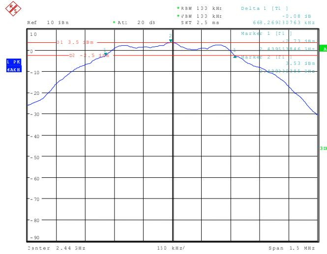
111592\_312.wmf: 6 dB bandwidth at the upper end of the assigned frequency band:
