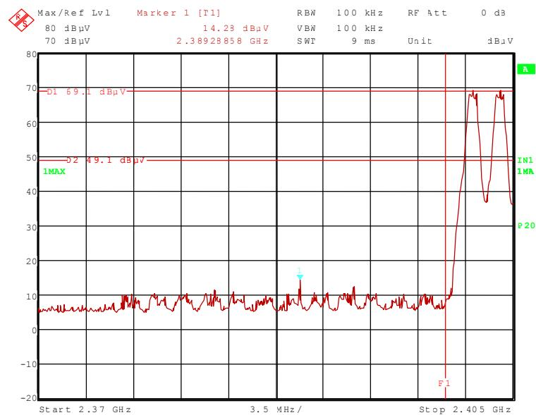
111592\_66.wmf: Radiated band-edge compliance, upper band edge, hopping off (operation mode 8):
