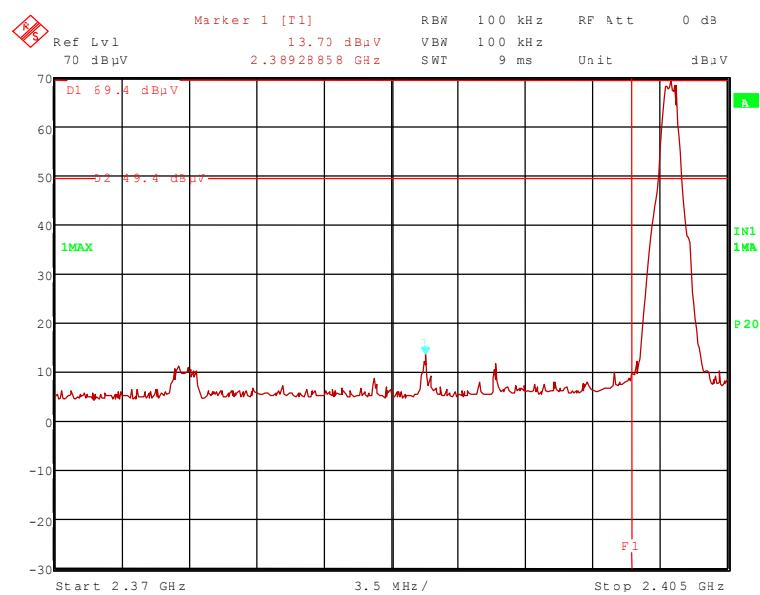
111592\_140.wmf: Radiated band-edge compliance, lower band edge, hopping on (operation mode 9):
