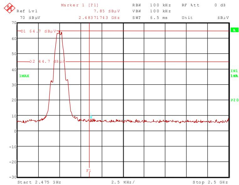
111592\_135.wmf: Radiated band-edge compliance, upper band edge, hopping on (operation mode 9):
