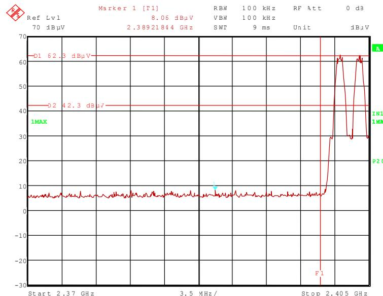
111592\_118.wmf: Radiated band-edge compliance, upper band edge, hopping off (operation mode 8):
