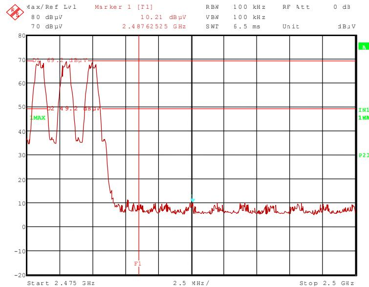
The plots on the page before are showing the radiated band-edge compliance for the upper band-edge, with and without hopping. The display line 1 (D1) in these plots represents the highest level within the assigned frequency band. The display line 2 (D2) represents the 20 dB offset to this highest level and shows the compliance with FCC 47 CFR Part 15.247 (d). The frequency line 1 (F1) shows the edge of the assigned frequency.
