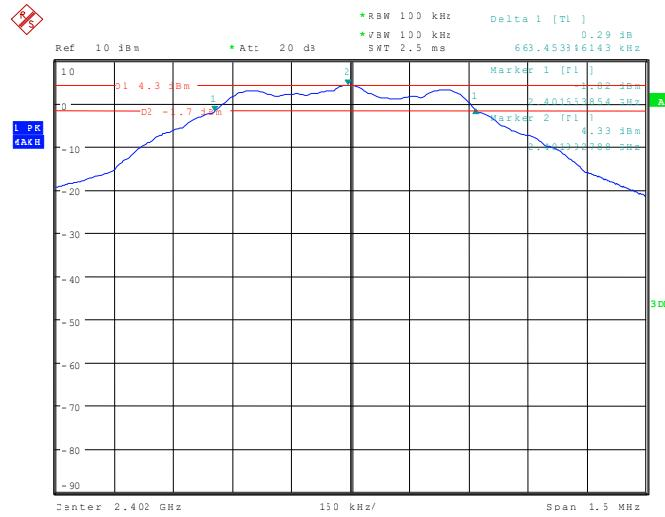
111592\_311.wmf: 6 dB bandwidth at the middle of the assigned frequency band:
