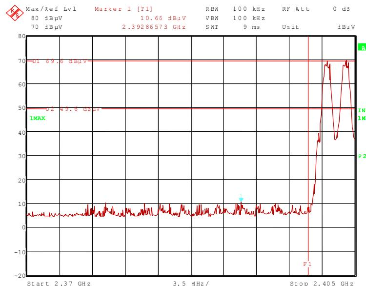
111592\_71.wmf: Radiated band-edge compliance, upper band edge, hopping off (operation mode 8):
