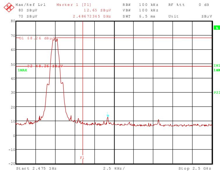
111592\_141.wmf: Radiated band-edge compliance, upper band edge, hopping on (operation mode 9):
