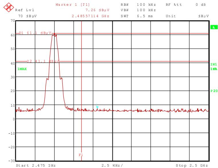
111592\_136.wmf: Radiated band-edge compliance, upper band edge, hopping on (operation mode 9):
