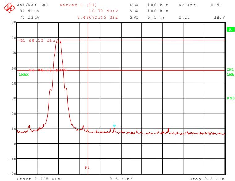
111592\_139.wmf: Radiated band-edge compliance, upper band edge, hopping on (operation mode 9):
