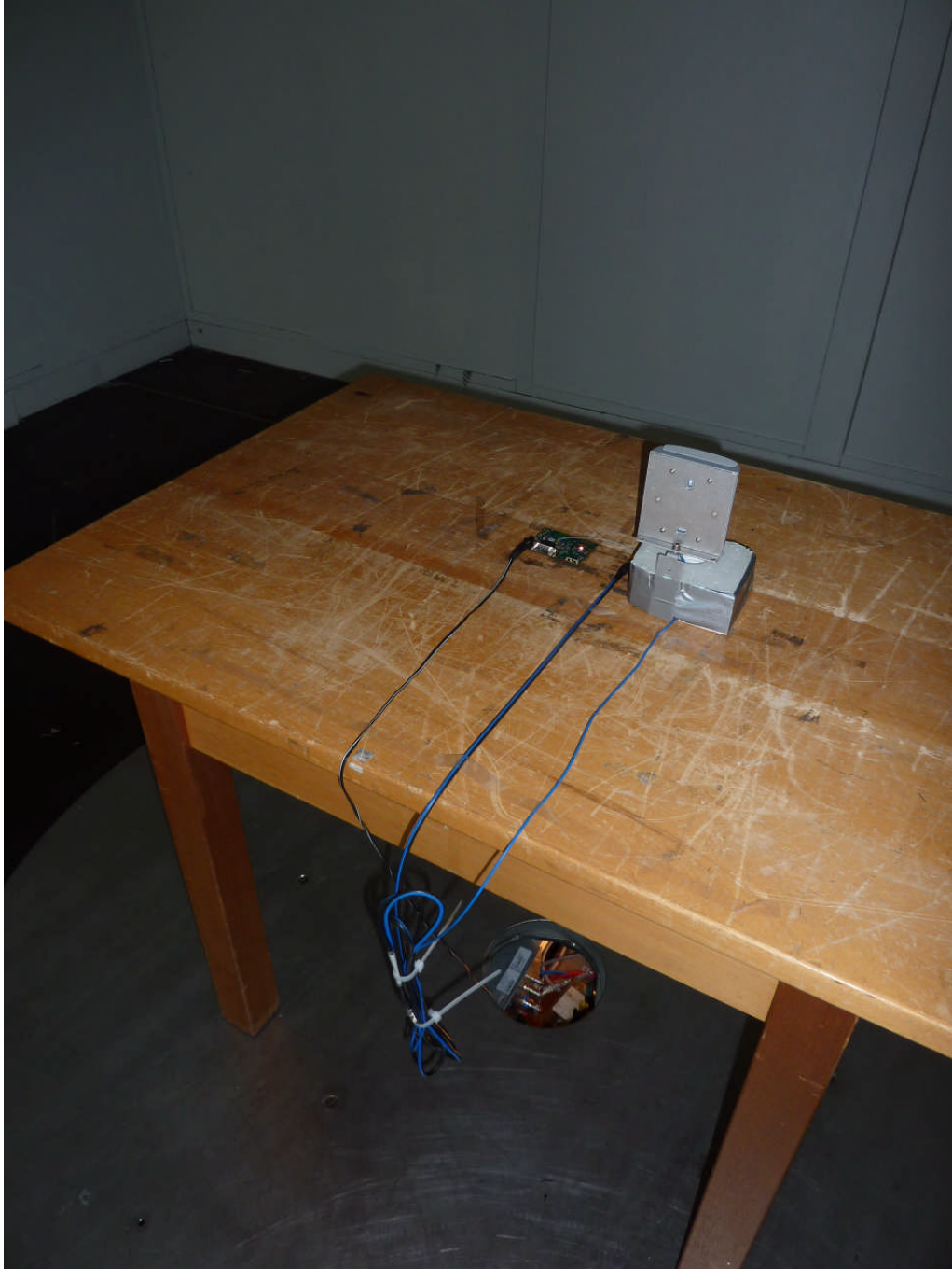
111592_33.JPG: cB-0946 with external patch antenna, test setup open area test site
