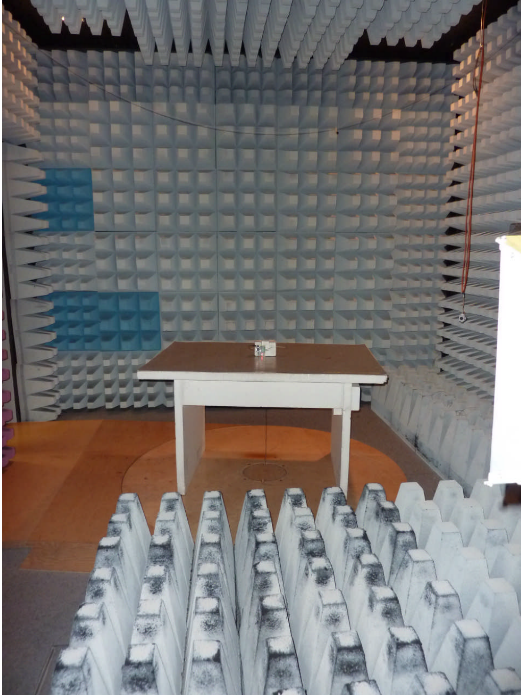
111592_2.JPG: cB-0946 with internal antenna, test setup fully anechoic chamber
