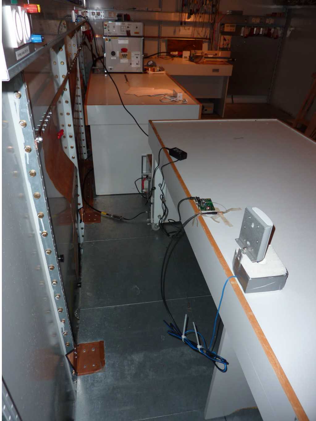
111592_35.JPG: cB-0946 with external patch antenna, test setup shielded chamber
