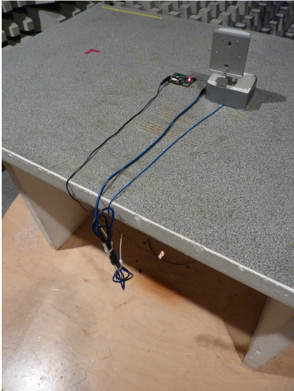
111592_4.JPG: cB-0946 with external patch antenna, test setup fully anechoic chamber (pos. 1)
