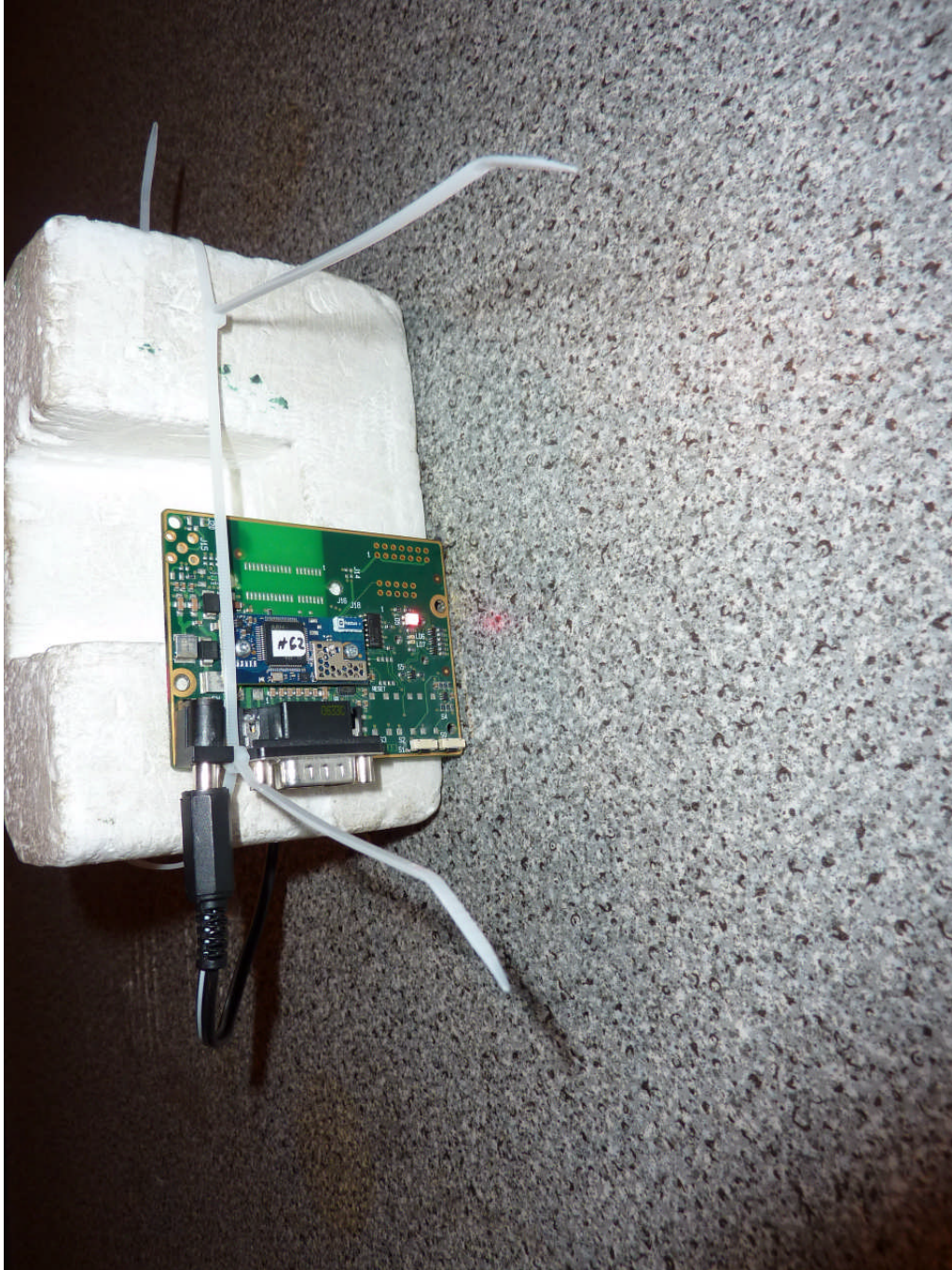
111592_1.JPG: cB-0946 with internal antenna, test setup fully anechoic chamber (pos. 2)
