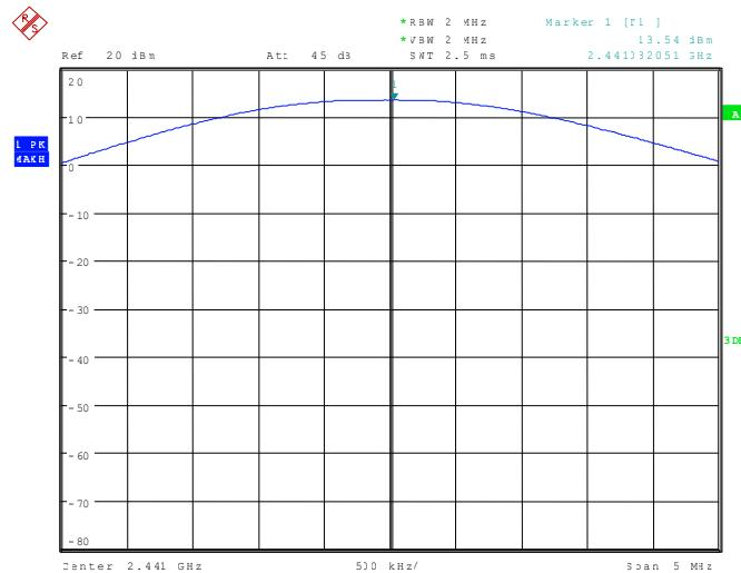
112117\_32.wmf: Maximum peak output power at the upper end of the assigned frequency band (operation mode 3):
