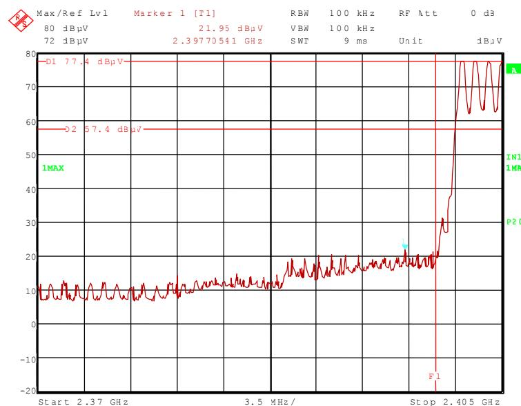
112117\_5.wmf: Radiated band-edge compliance, upper band edge, hopping off (operation mode 3):
