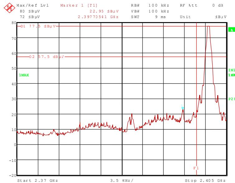
112117\_7.wmf: Radiated band-edge compliance, lower band edge, hopping on (operation mode 4):
