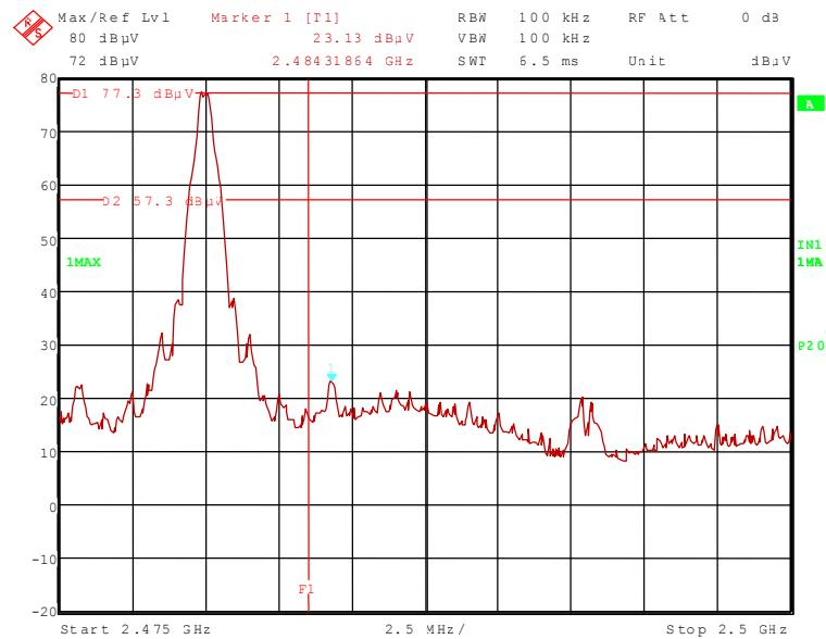
112117\_6.wmf: Radiated band-edge compliance, upper band edge, hopping on (operation mode 4):
