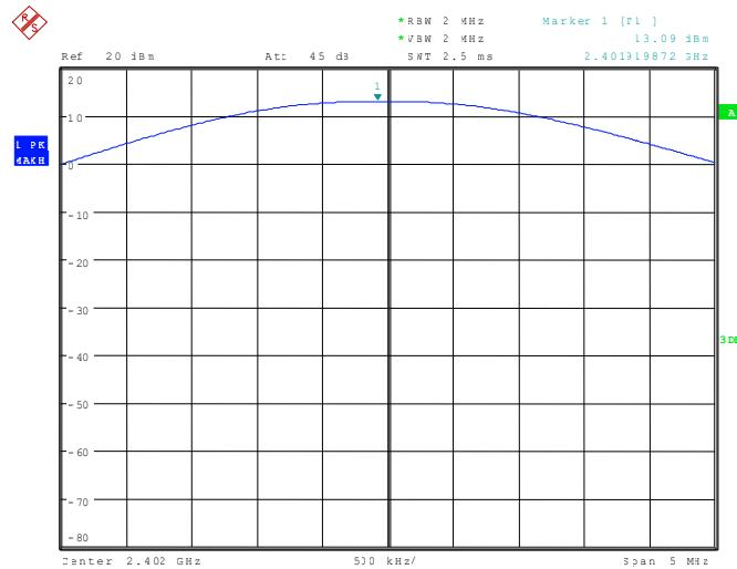
112117\_31.wmf: Maximum peak output power at the middle of the assigned frequency band (operation mode 2):
