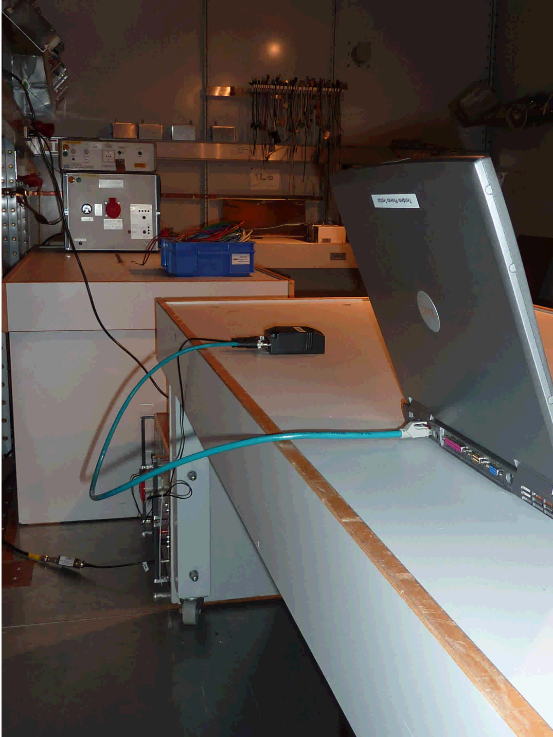
101042_23.jpg cB-RWE231, test set-up conducted emission measurement
