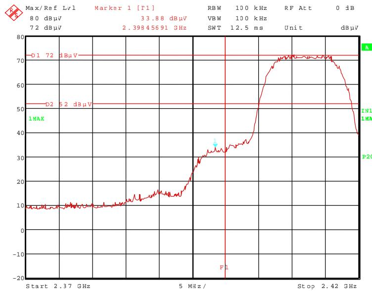
101042\_4.wmf: Radiated band-edge compliance, upper band edge, b-mode, 11 Mbps:
