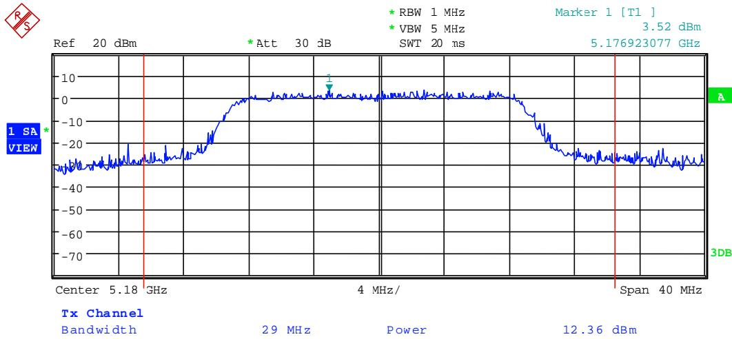
91568\_261.wmf: Maximum conducted output power, operation mode 2, n-mode, 6 Mbps:
