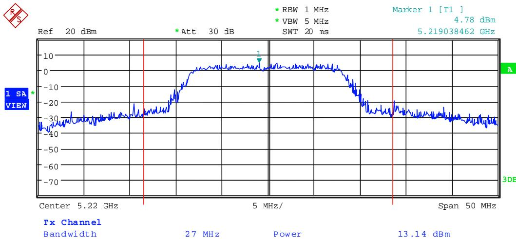
91568 266.wmf: Maximum conducted output power, operation mode 4, a-mode, 6 Mbps:
