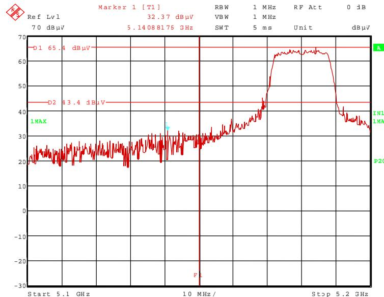
91568\_451.wmf: Radiated band-edge compliance, operation mode 4, a-mode, 54 Mbps:
