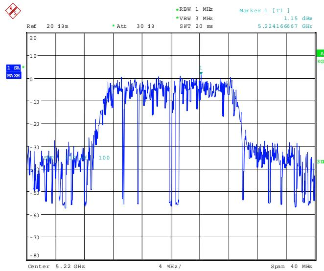
91568\_274.wmf: Peak power spectral density, operation mode 4, n-mode, 6 Mbps:
