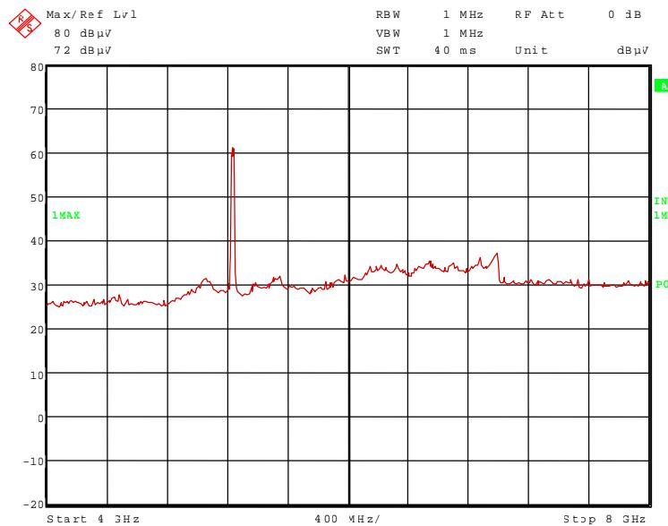
91568\_465.wmf: Spurious emissions from 8 GHz to 12 GHz (n-mode, 6 Mbps, operation mode 4):
