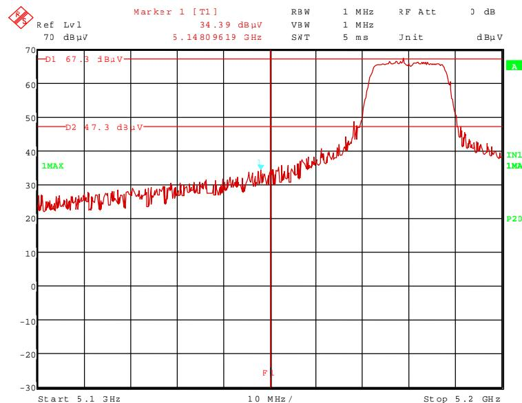
91568\_36.wmf: Radiated band-edge compliance, operation mode 4, a-mode, 54 Mbps:
