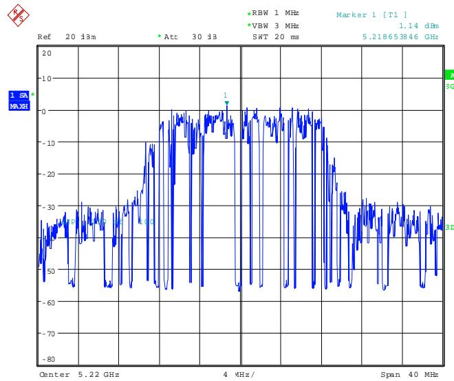
91568\_267.wmf: Peak power spectral density, operation mode 4, a-mode, 6 Mbps:
