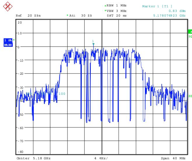
91568\_272.wmf: Peak power spectral density, operation mode 2, n-mode, 6 Mbps:
