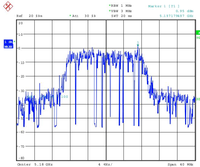
91568\_269.wmf: Peak power spectral density, operation mode 2, a-mode, 6 Mbps:
