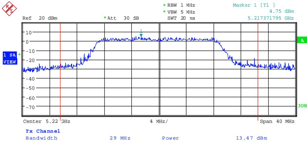
91568 259.wmf: Maximum conducted output power, operation mode 4, n-mode, 6 Mbps:
