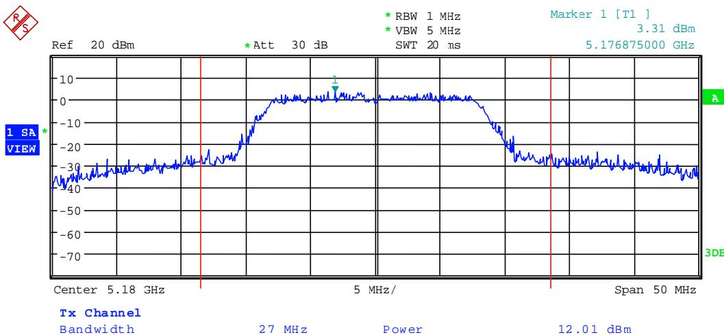
91568\_264.wmf: Maximum conducted output power, operation mode 2, a-mode, 6 Mbps:
