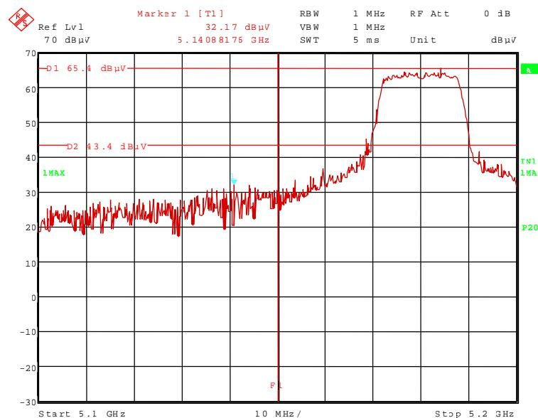
91568\_144.wmf: Radiated band-edge compliance, operation mode 4, a-mode, 54 Mbps:
