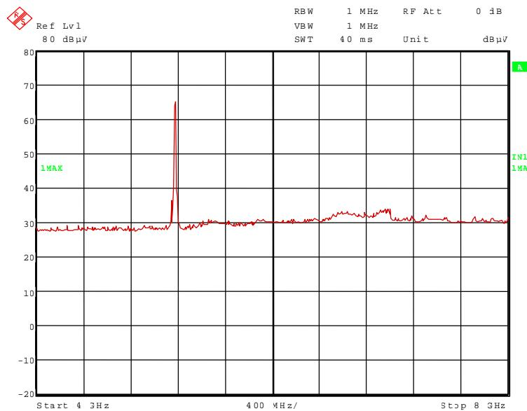
91568\_33.wmf: Spurious emissions from 8 GHz to 12 GHz (a-mode, 6 Mbps):
