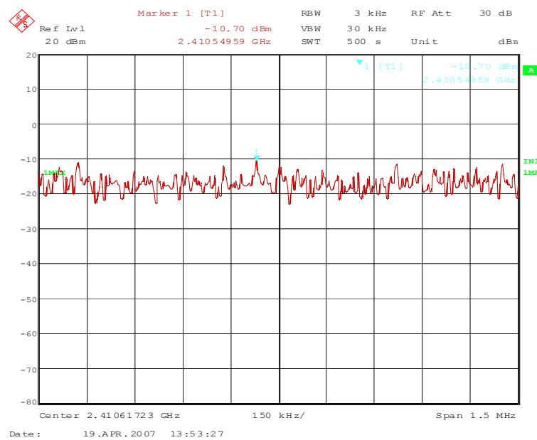
70284\_39.wmf (power spectral density (transmit on channel 6), operation mode 2):
