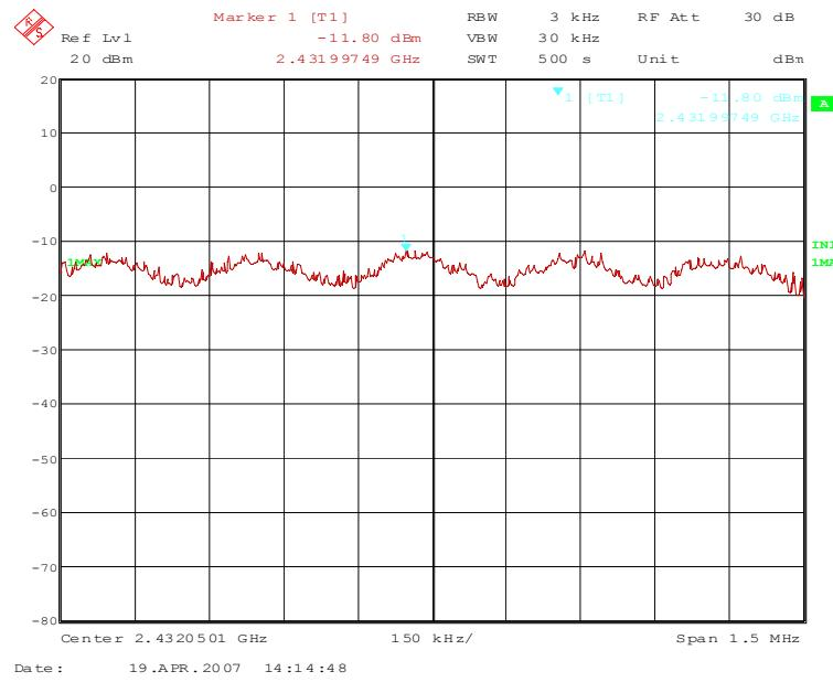
**70284\_42.wmf (power spectral density (transmit on channel 11), operation mode 6):**
