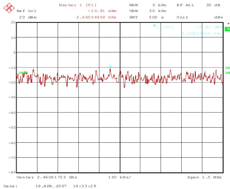
**70284\_38.wmf (power spectral density (transmit on channel 1), operation mode 4):**
