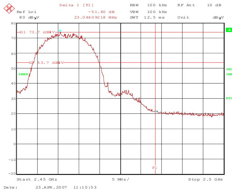
70284\_69.wmf (radiated band-edge compliance, lower band edge, operation mode 1):
