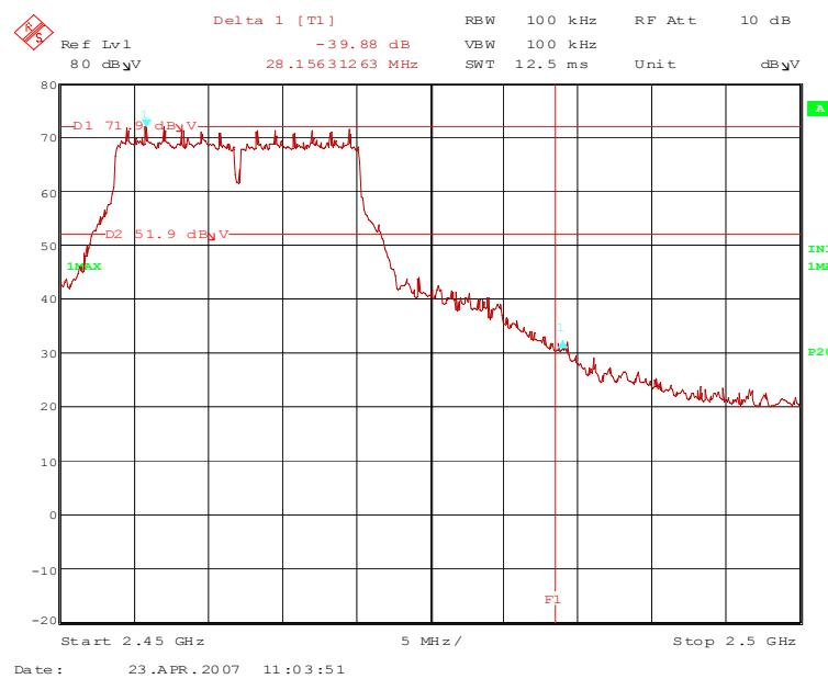
70284\_70.wmf (radiated band-edge compliance, lower band edge, operation mode 4):
