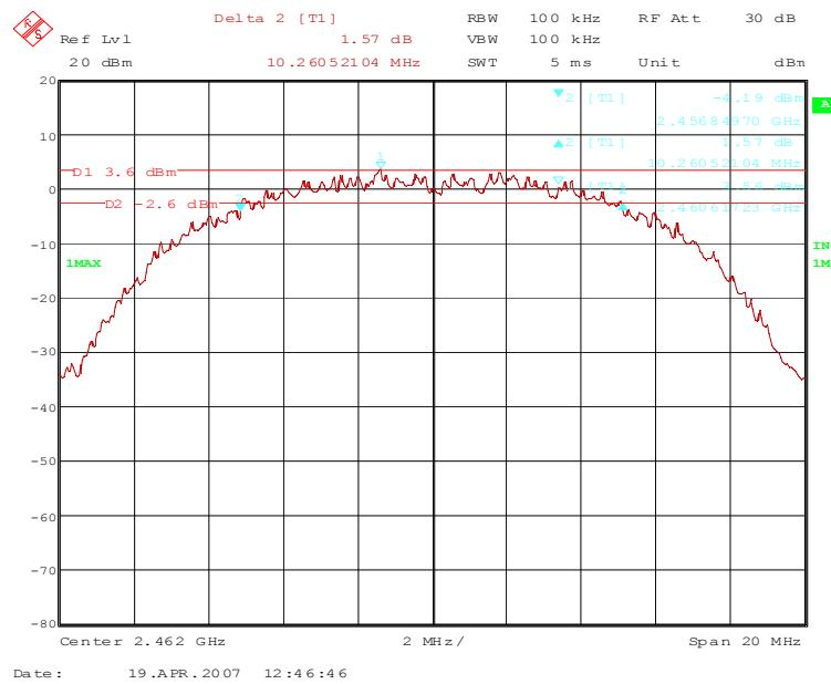
**70284\_32.wmf: (6 dB bandwidth at the lower end of the assigned frequency band, operation mode 4):**
