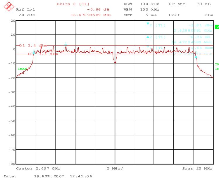
**70284\_36.wmf: (6 dB bandwidth at the upper end of the assigned frequency band, operation mode 6):**
