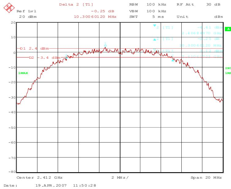
70284\_33.wmf: (6 dB bandwidth at the middle of the assigned frequency band, operation mode 2):
