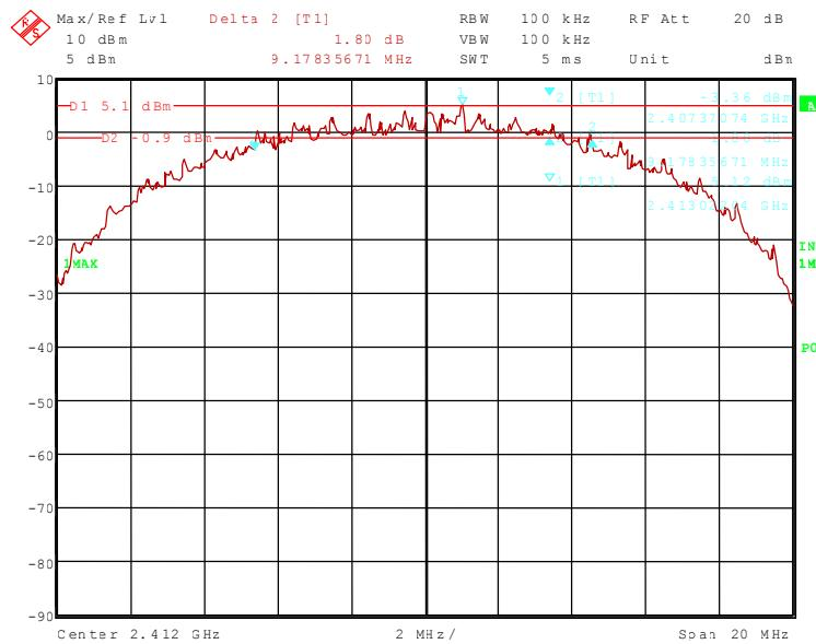
60502\_66.wmf: (6 dB bandwidth at the middle of the assigned frequency band):
