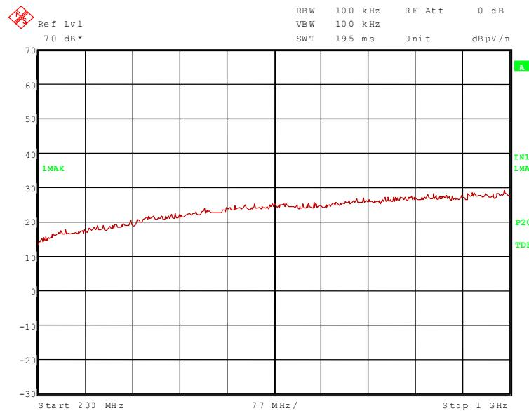
No significant emissions above the noise floor found during the preliminary emission test. So no final test has to be carried out on an open area test site.
