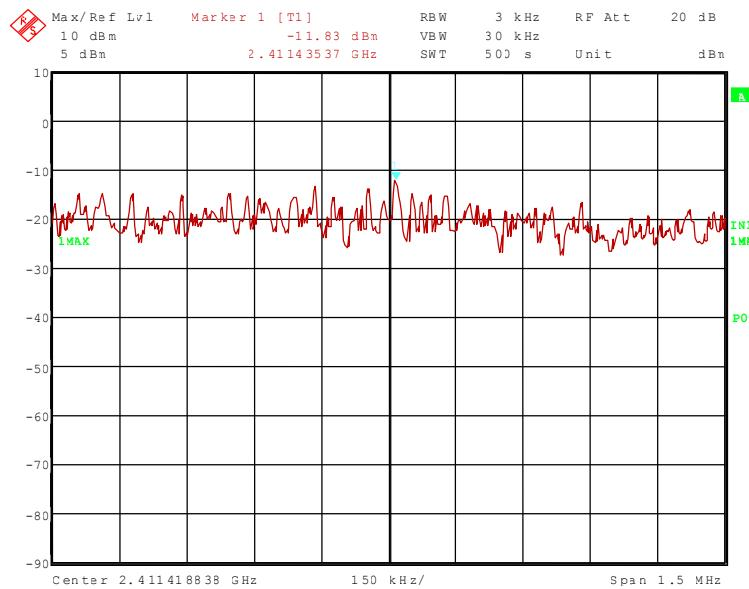
60502\_61.wmf (power spectral density (transmit on channel 6)):
