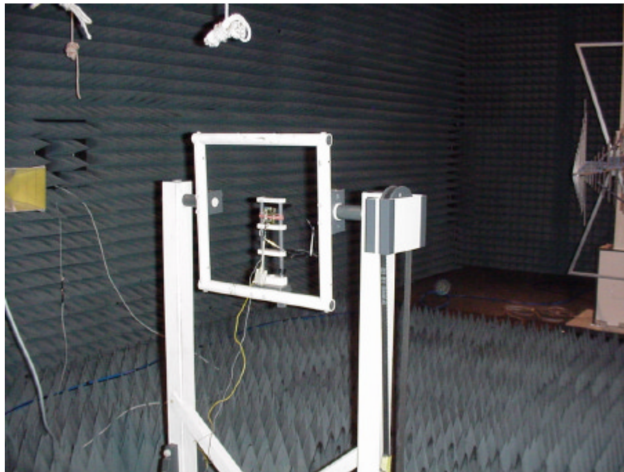
Picture 3 : Setup for radiated emission tests
