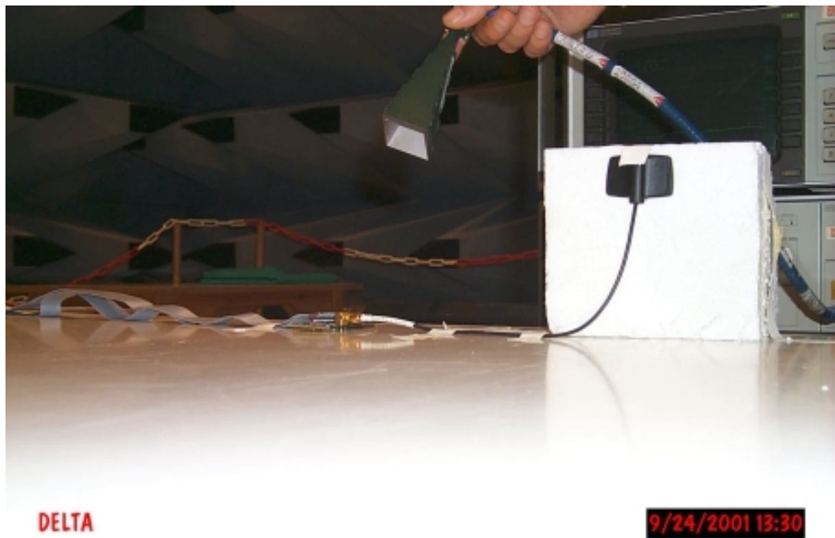
PHOTO A2.5 Test set-up for test 18-26 GHz
