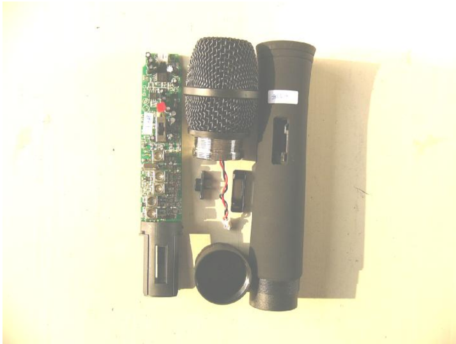
Tx Main board component side
