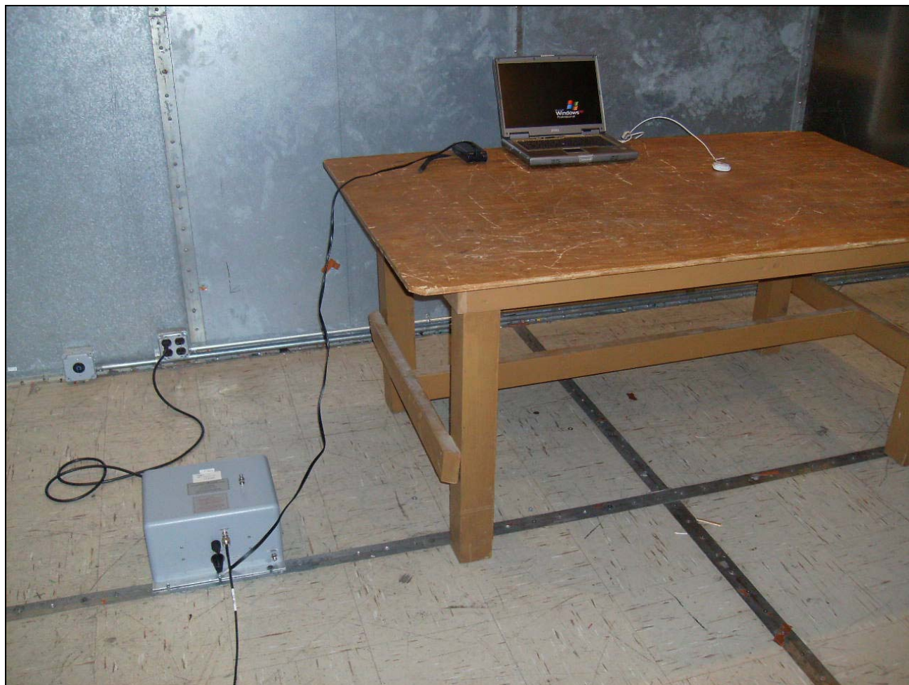
Photograph 1. Conducted Emissions Test Setup
