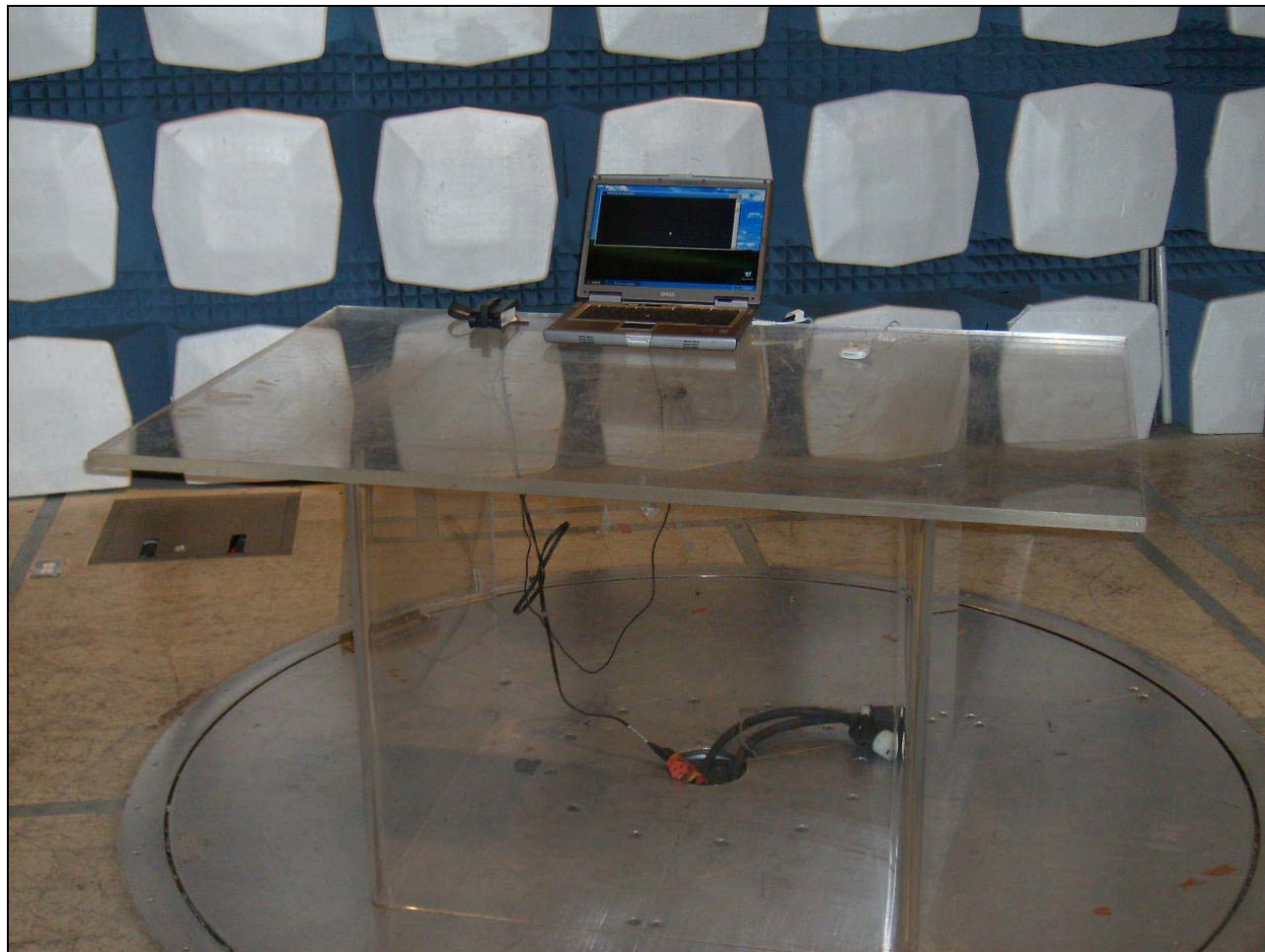
Photograph 2. Radiated Emission Limits Test Setup
