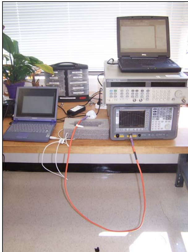
Photograph 7. Peak Power Spectral Density Test Setup
