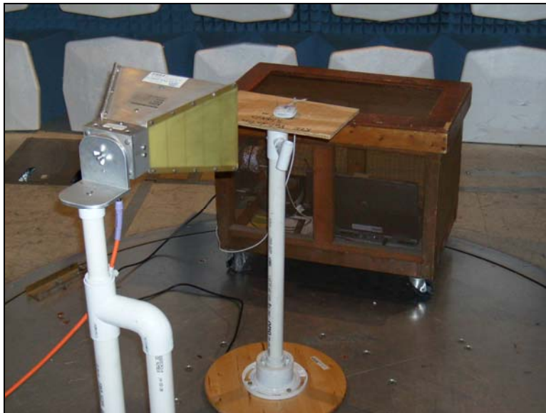
Photograph 3. Spurious Radiated Emissions, Test Setup
