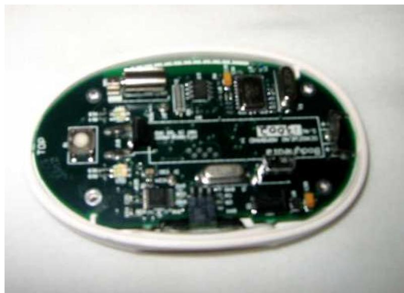
Install the main PCB by sliding into the HF PCB connector and then lowering into place. Make sure the two PCB notches align with the ribs in the bottom plastic.
