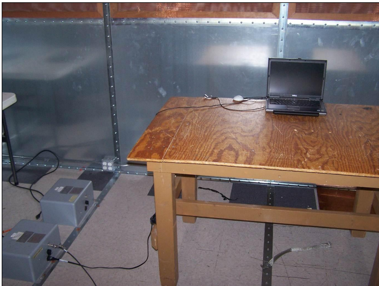
Photograph 1. Conducted Emissions, Test Setup
