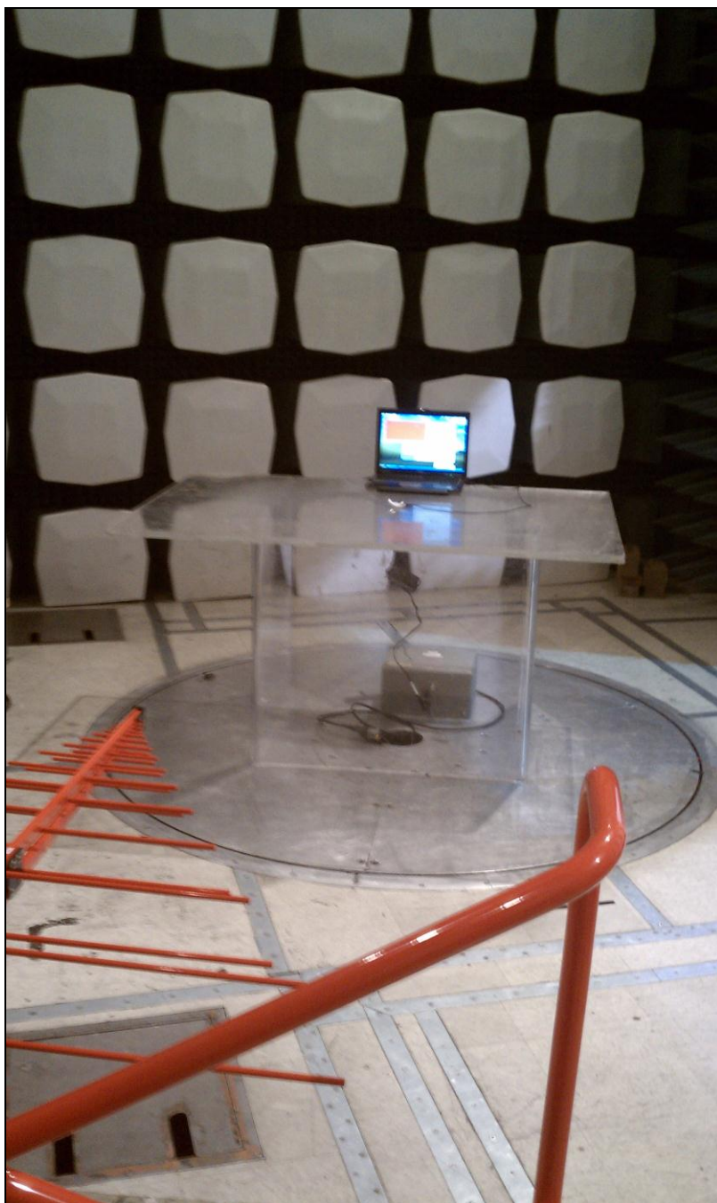
Photograph 3. Radiated Emission Limits Test Setup
