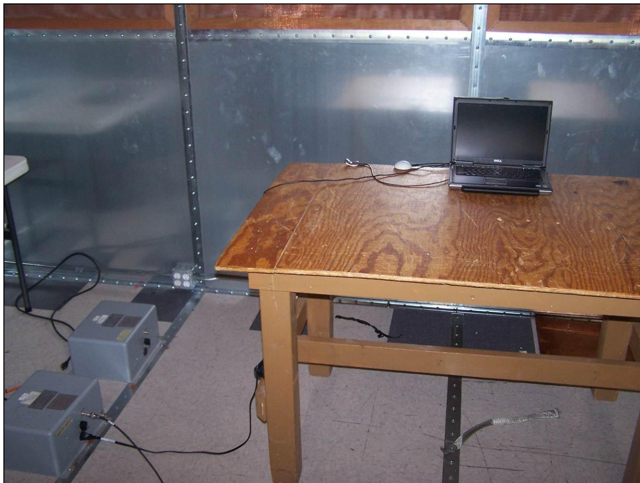
Photograph 2. Conducted Emissions Test Setup
