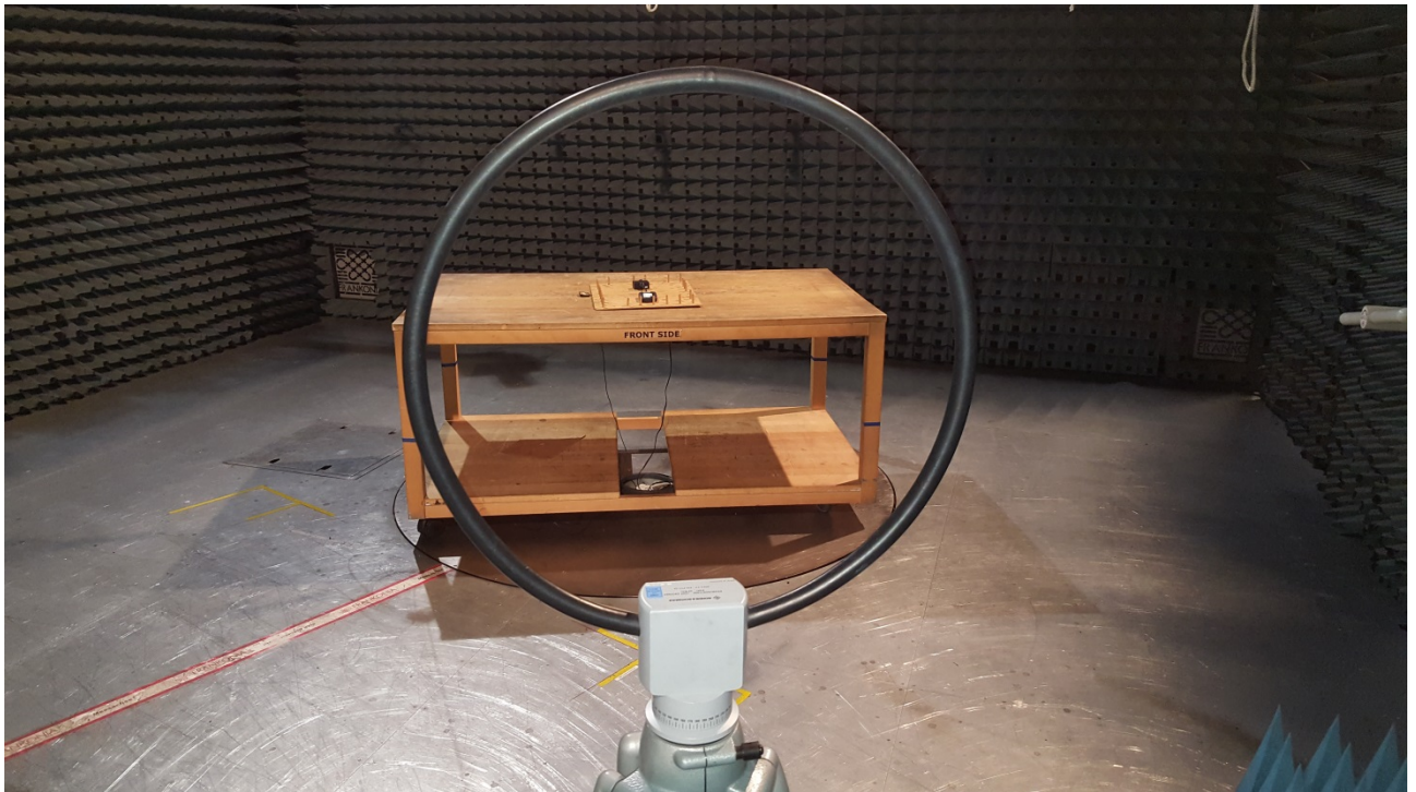
Photo 1: Test setup for radiated measurements below 30 MHz, front side view
