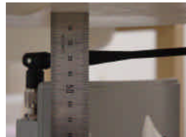
Fig. 21. Body SAR Test Setup with Holster
