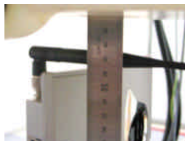
Fig. 21. Body SAR Test Setup with Holster
