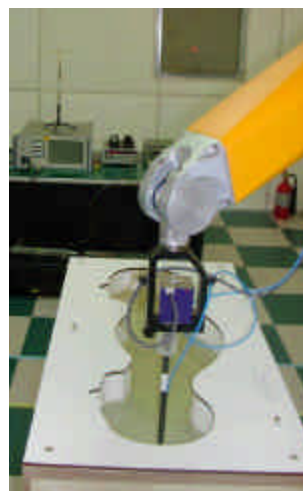
Figure 4. Photograph of the probe and the Phantom
