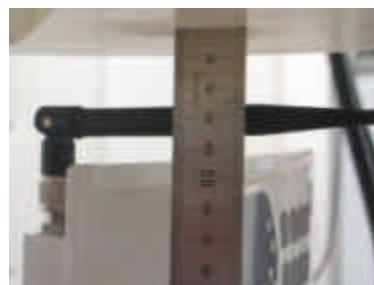
Fig. 21. Body SAR Test Setup with Holster
