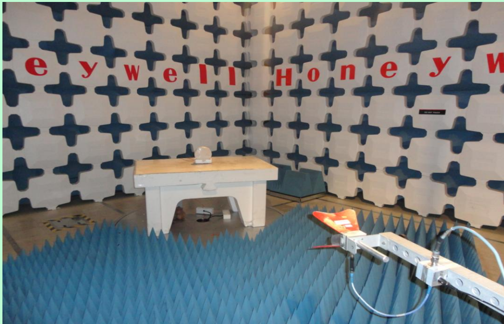
Radiated Emission Setup – 1 GHz to 10 GHz [ Vertical ]
