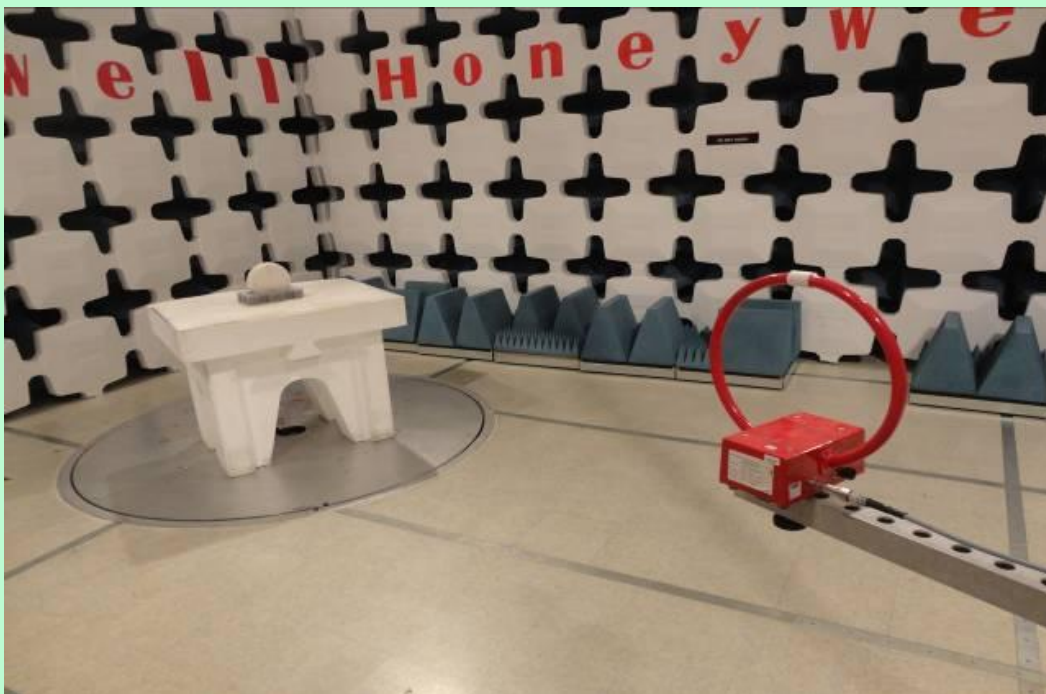
Radiated Emission Setup – 9 KHz to 30 MHz [ Perpendicular ]
