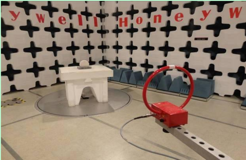
Radiated Emission Setup – 9 KHz to 30 MHz [ Parallel ]
