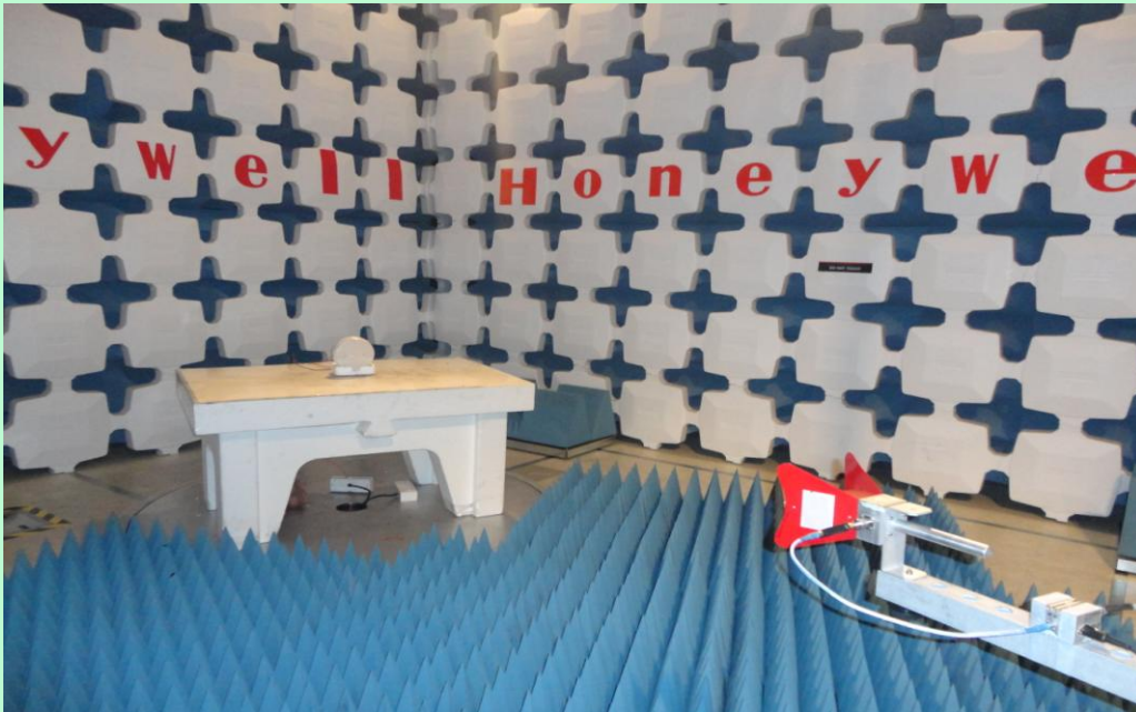
Radiated Emission Setup – 1 GHz to 10 GHz [ Horizontal ]
