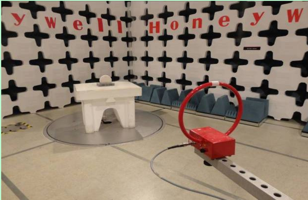
Radiated Emission Setup – 9 KHz to 30 MHz [ Parallel ]
