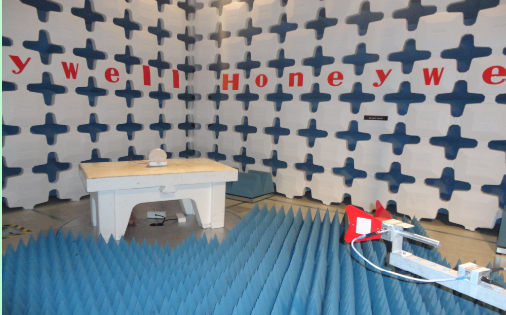
Radiated Emission Setup – 1 GHz to 10 GHz [ Horizontal ]
