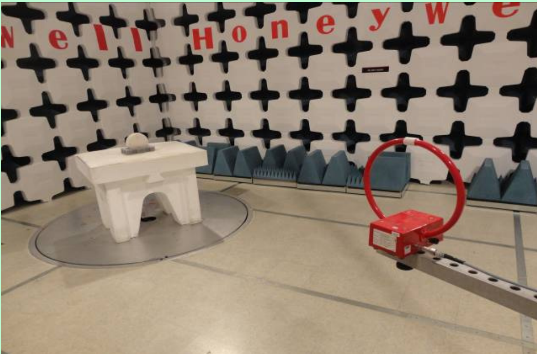
Radiated Emission Setup – 9 KHz to 30 MHz [ Perpendicular ]
