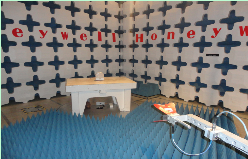
Radiated Emission Setup – 1 GHz to 10 GHz [ Vertical ]
