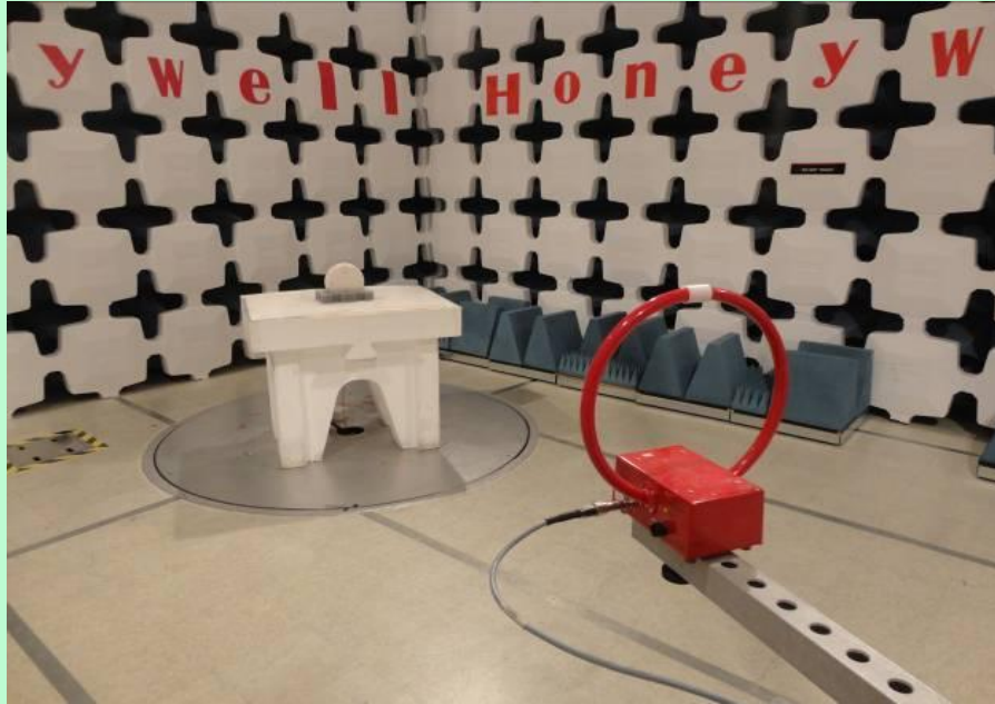
Radiated Emission Setup – 9 KHz to 30 MHz [ Parallel ]
