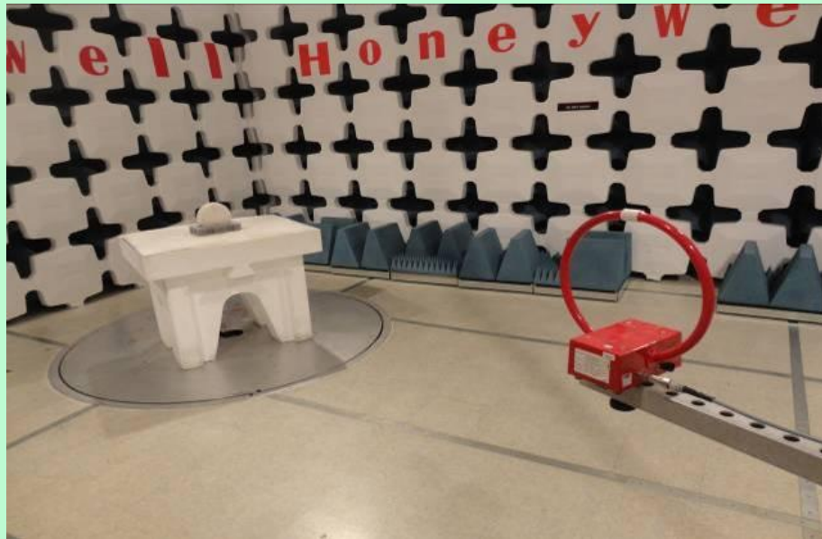
Radiated Emission Setup – 9 KHz to 30 MHz [ Perpendicular ]
