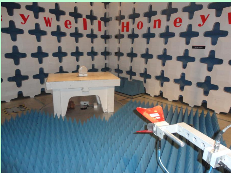
Radiated Emission Setup – 1 GHz to 10 GHz [ Perpendicular Polarization ]
