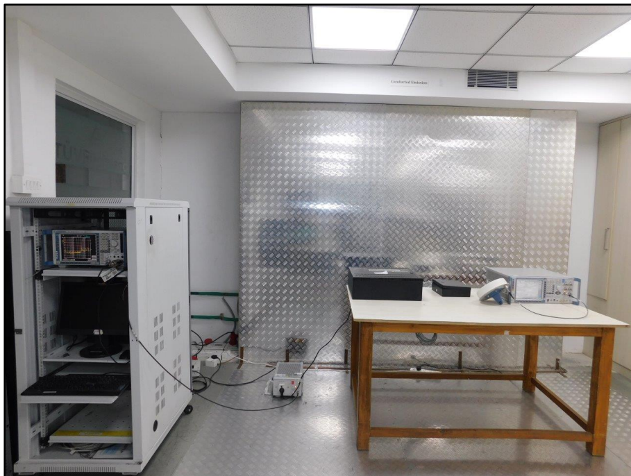
Conducted Emission Setup Photo
