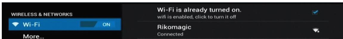
When opened the WIFI, the MK802 IV will auto search available wireless router signals within 20 meters, user just choose a router and input correct password to connected network.
