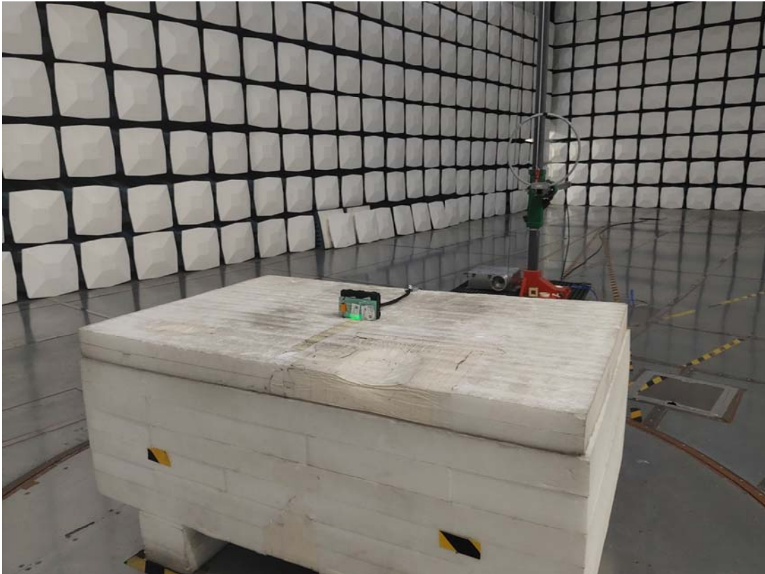
Radiated Emission 9k-30MHz Perpendicular View
