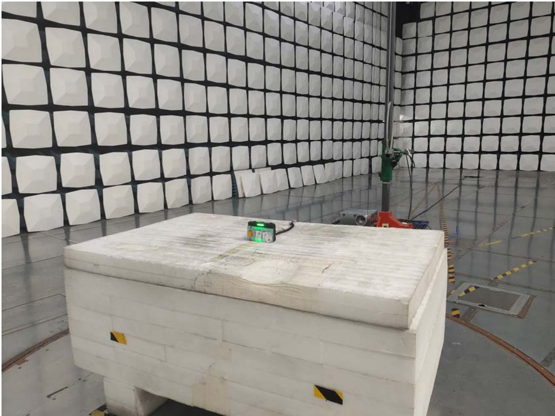
Radiated Emission 9k-30MHz Perpendicular View
