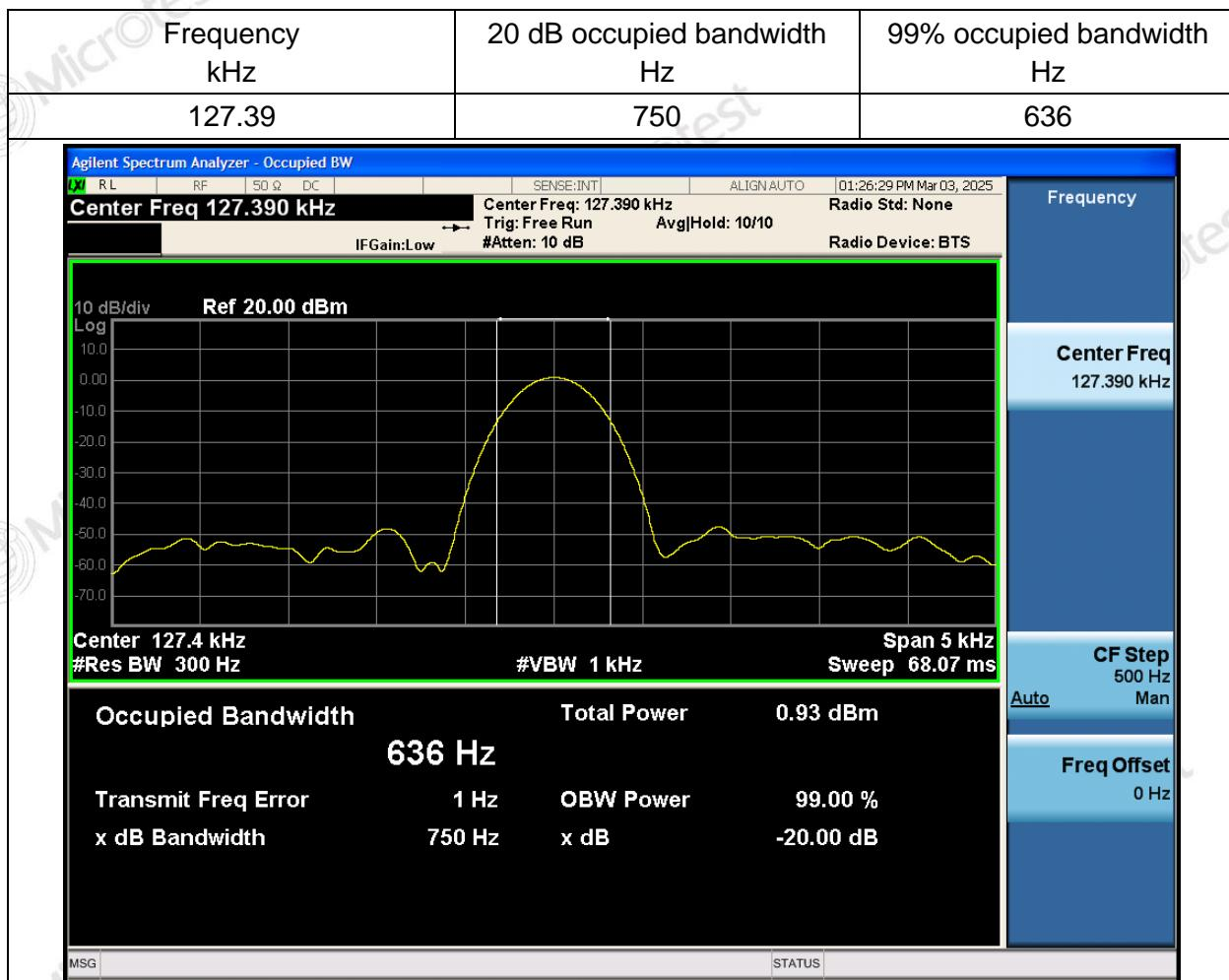
**Note:** Because the measured signal is CW-like, adjusting the RBW per C63.10 would not be practical since measurement bandwidth will always follow the RBW. The RBW is set to 300 Hz to perform the occupied bandwidth test.
