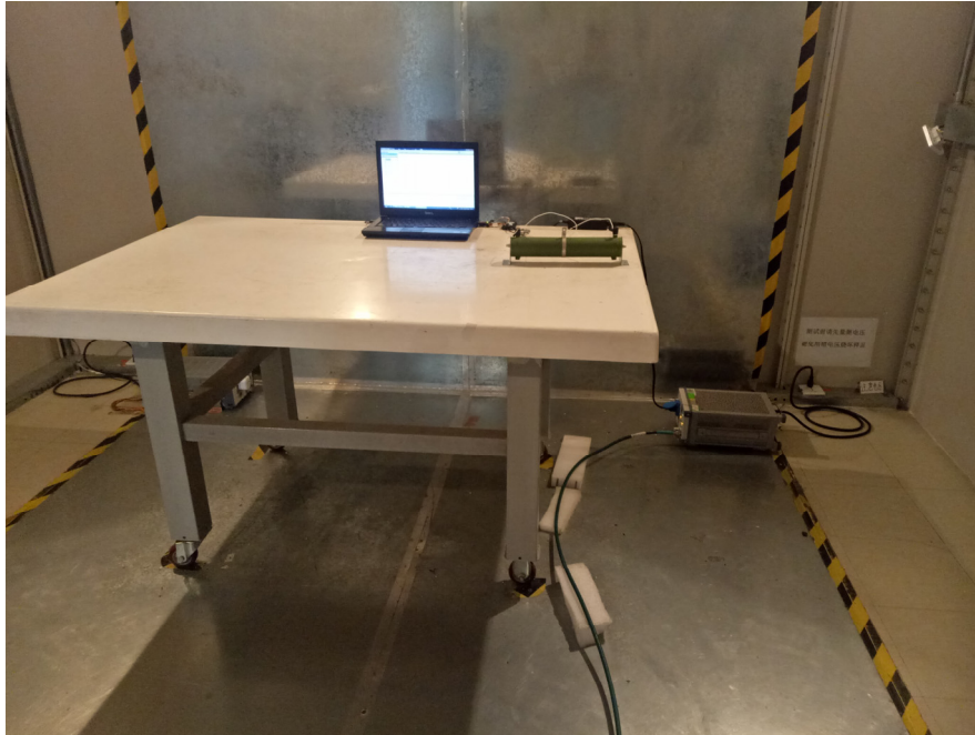
Conducted Emissions (Side View)
