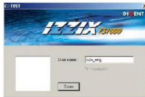
⑤ Put your finger on the Fingerprint Identification Device and click [Scan] button to view the folder.
