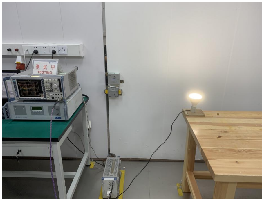
Conducted Emissions Test Setup
