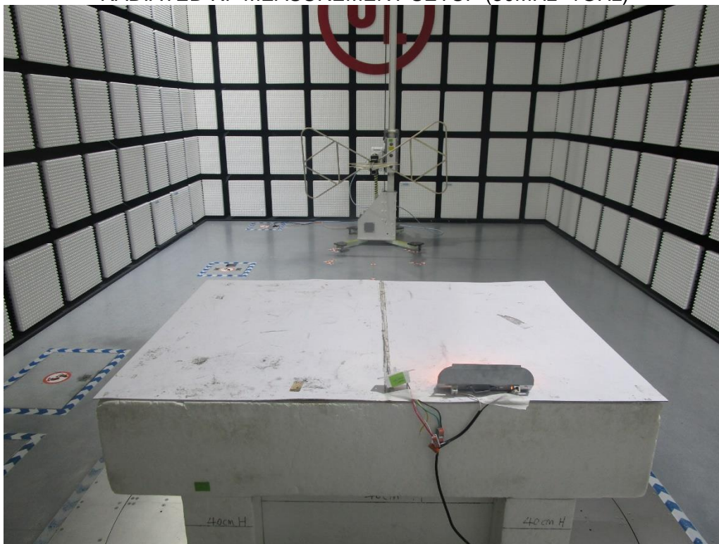
RADIATED RF MEASUREMENT SETUP (Below 30MHz)
