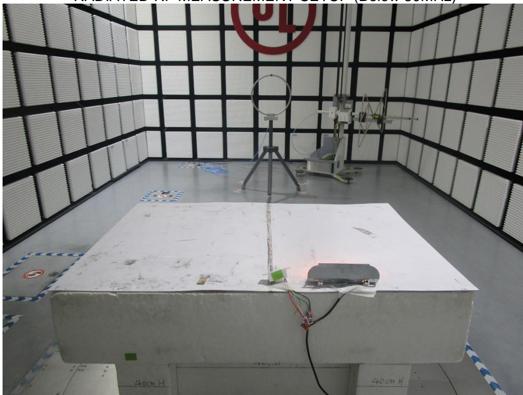
RADIATED RF MEASUREMENT SETUP (Below 30MHz)
