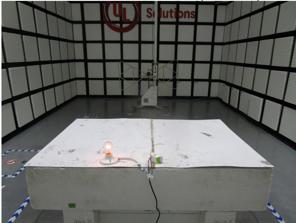
RADIATED RF MEASUREMENT SETUP (Below 30MHz)
