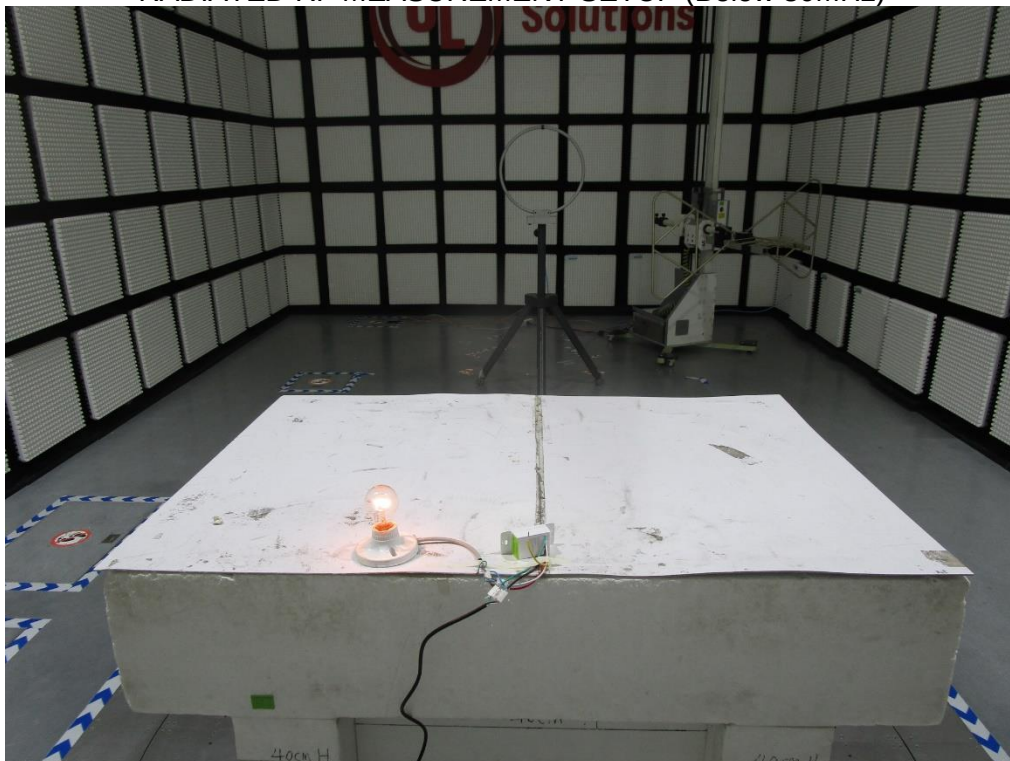
RADIATED RF MEASUREMENT SETUP (Below 30MHz)
