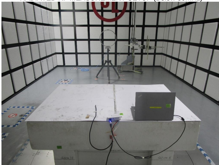
RADIATED RF MEASUREMENT SETUP (Below 30MHz)
