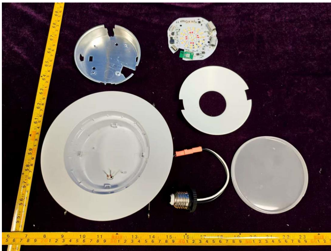
FIGURE 7 DOWNLIGHT (CFIXRSCR6CRVDMS) COVER REMOVE
