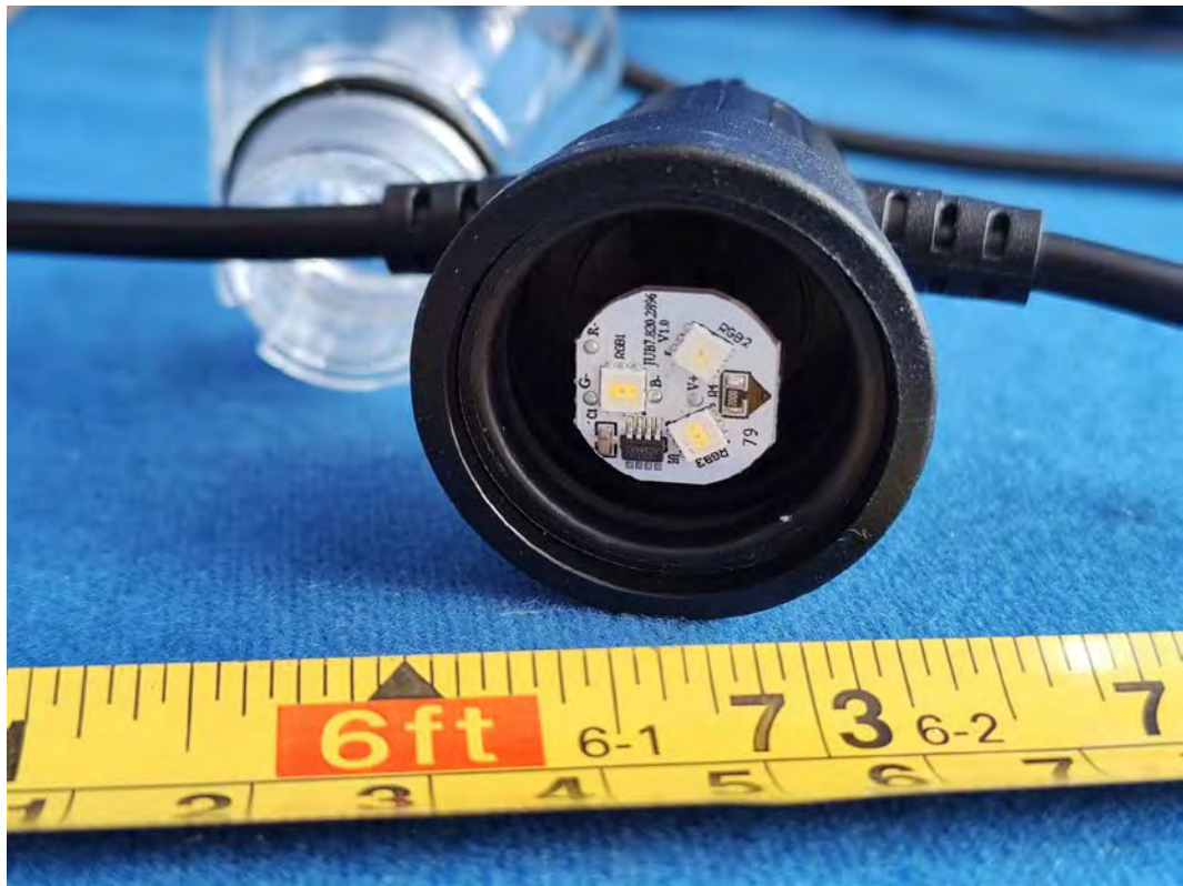
FIGURE 39 CYNIC DYNAMIC EFFECTS SMART CAFÉ LIGHTS (M/N: CCF96CDOD/ENS) BULB COVER REMOVE
