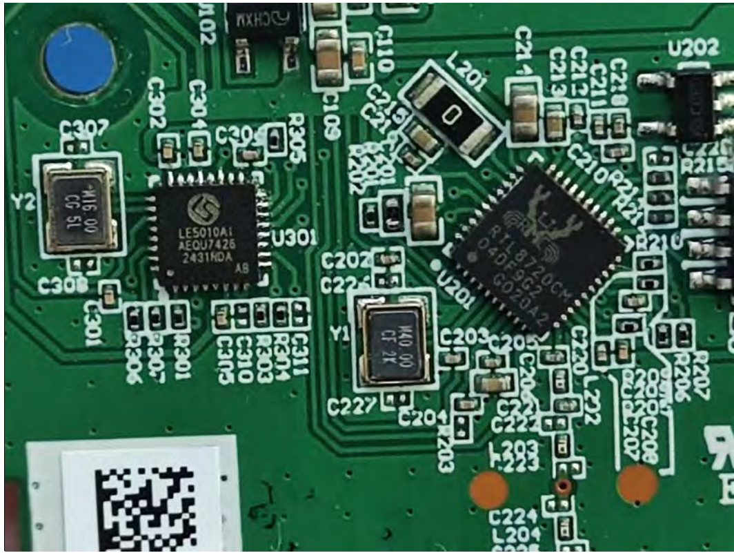
FIGURE 30 CYNIC DYNAMIC EFFECTS SMART CAFÉ LIGHTS (M/N: CCF24CDOD/ENS) CHIP&CRYSTAL ON BOARD
